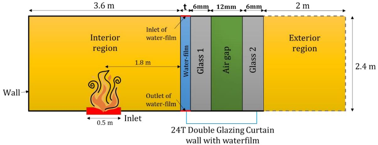
Fig. 1. Schematic of the numerical domain
