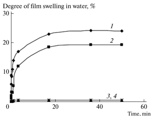
Fig. 3. Kinetics of swelling of (1–2) LDPE films with sulfonation degrees of  $CA^{\text{SO}_3\text{H}} = 5.8 \times 10^{-3}$  and (2)  $2.1 \times 10^{-3}$  kg/m<sup>2</sup>, (3) the pristine LDPE film, and (4) the successively fluorinated ( $CA^{\text{F}} = 4.7 \times 10^{-4}$  kg/m<sup>2</sup>) and sulfonated ( $CA^{\text{SO}_3\text{H}} = 1.1 \times 10^{-4}$  kg/m<sup>2</sup>) LDPE film in water.
