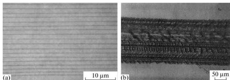
Fig. 2. Images of fluorinated LDPE films obtained on a POLAM R-312 optical polarization microscope: (a) with bands made by steel needles with subsequent sulfonation, no magnification; (b) with a sulfonated band, 50× magnification. The sulfonated bands of the pristine polymer are dark.
