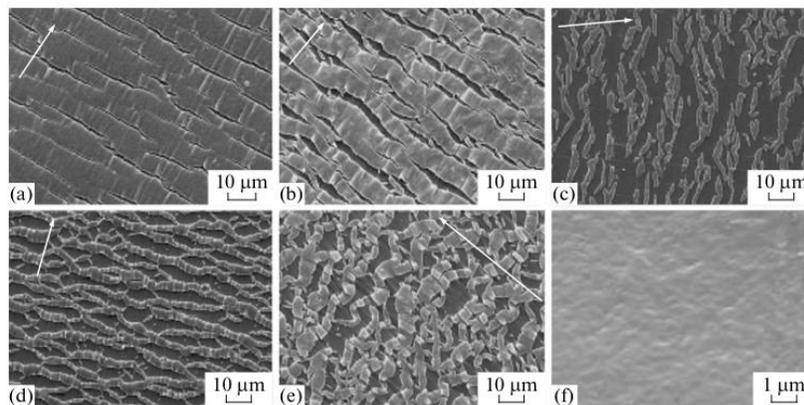
Fig. 1. Surface images of various films: (a) LDPE, (b) HDPE, (c) PET, and (d) PP fluorinated for 0.5 h and then stretched by 100%; (e) fluorinated HDPE after stretching by 200%; (f) fluorinated LDPE before stretching. Arrows indicate the stretching directions.
