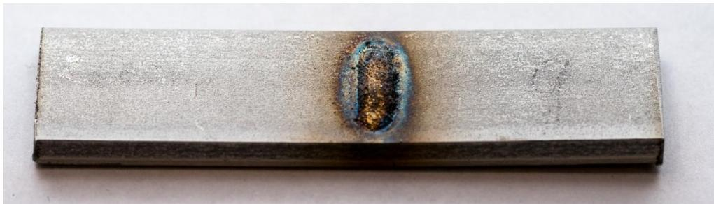
Fig. 1. A metal deposition process may produce nonuniform thermal expansion and contraction, resulting in distribution of residual stresses in the heat affect zone.
