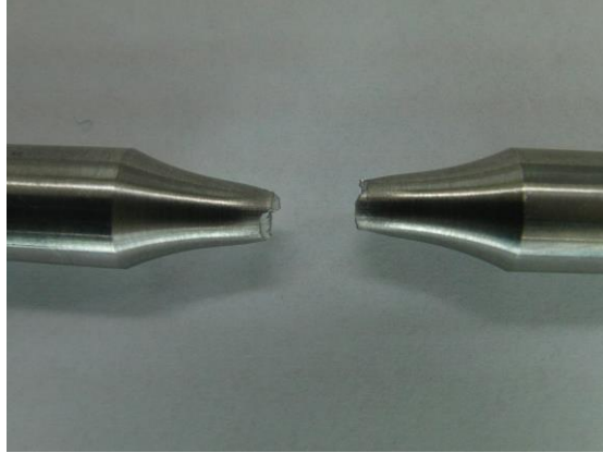
Fig. 2. Titanium alloy Ti6Al4V specimen after tensile testing
