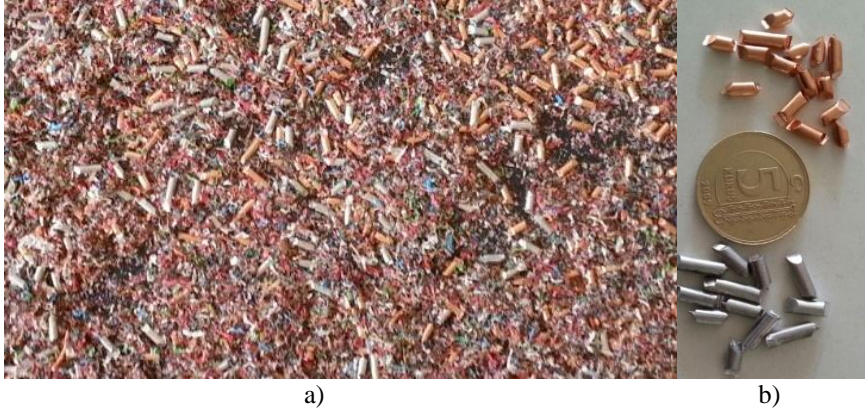
Fig. 3. Granule cable waste a) mixture cable waste with pvc b) granule cable
