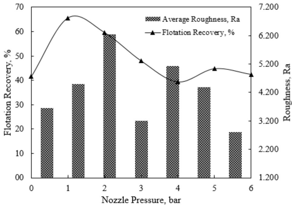
Fig. 5. Correlation between average roughness and flotation recoveries as a function of nozzle pressure
