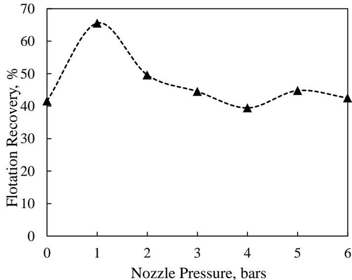
Fig. 2. Flotation recoveries as a function of nozzle pressure bar.
