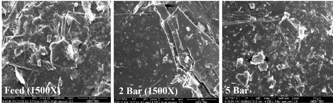
Fig. 3. SEM images of the samples (a) Un-blasted sample (1500X magnification) (b) blasted sample at 2 bars (1500X magnification) (c) blasted sample at 5 bars (1500X magnification)
