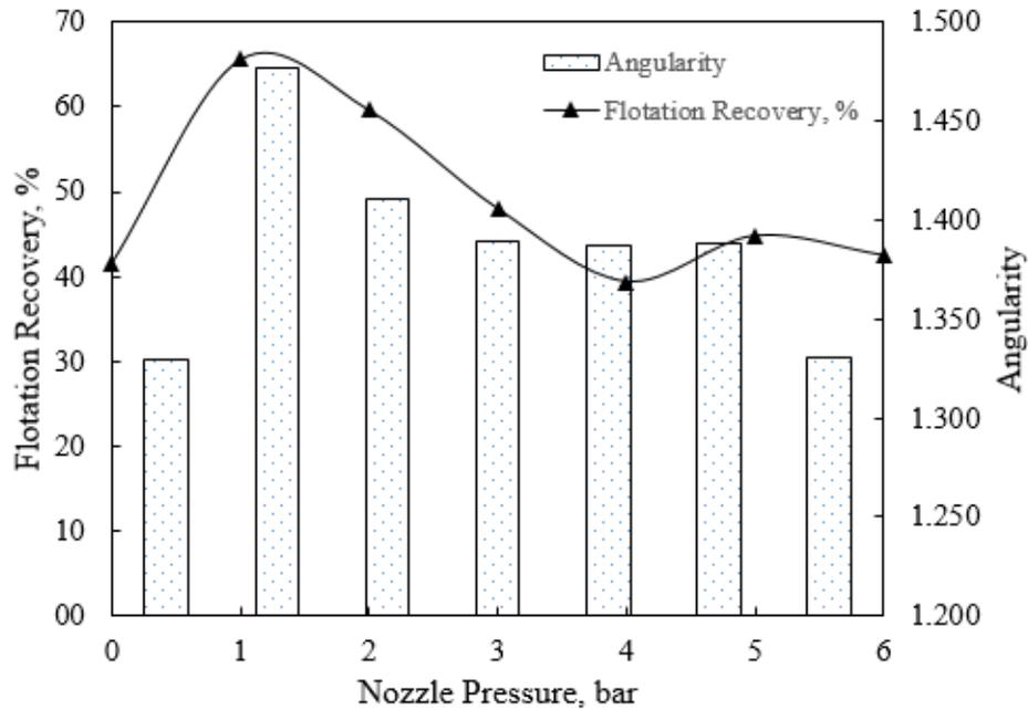
Fig. 4. The correlation between angularity and flotation recoveries as a function of nozzle pressures
