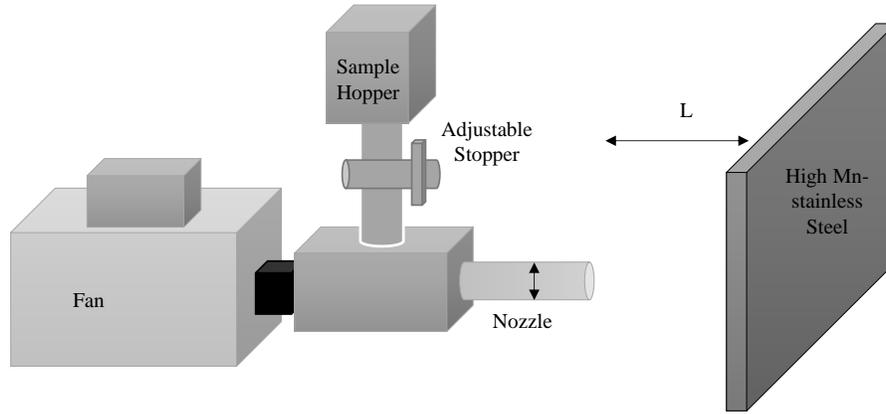
Fig. 1. Schematic illustration of the sand blasting equipment and orientation of plate
