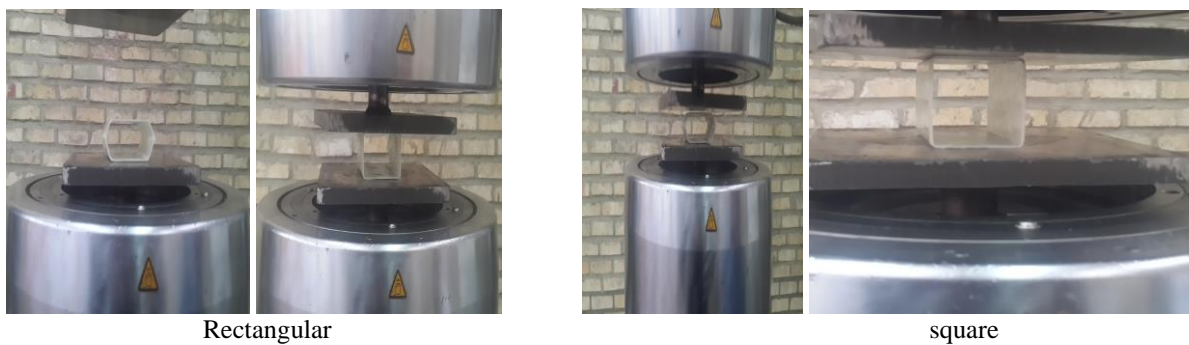
Fig. 6. Samples with rectangular and square tubes under loading Right: before loading left: after loading
