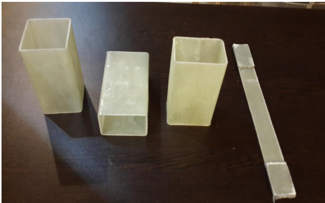
Fig. 1. prepared samples with different sections for performing experiments
