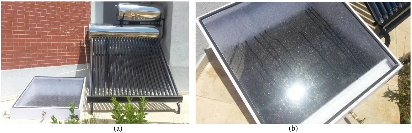
Fig. 2: Experimental setup a) An overview from the experimental setup; b) A view from the experiments (Evaporation and condensation processes in the main tank).
