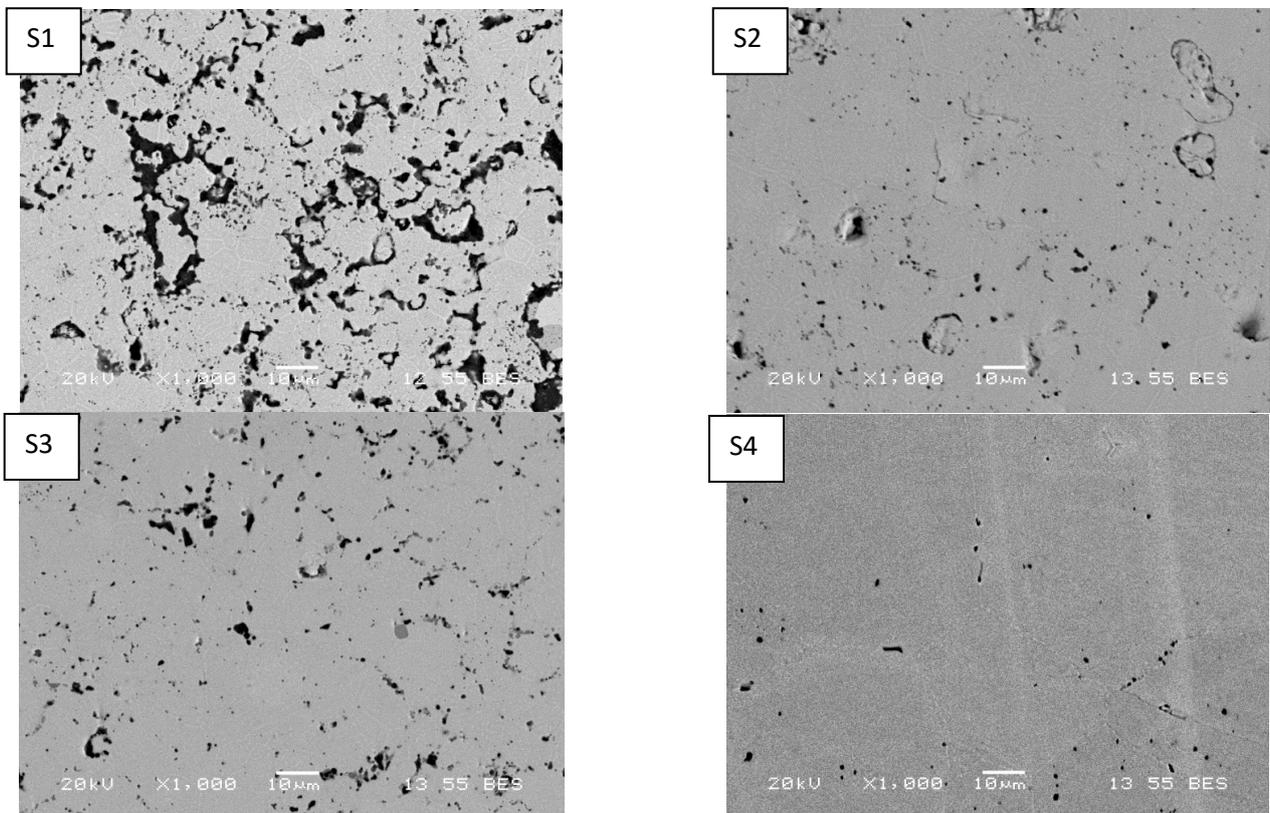
Fig. 2: Microstructure of CrNiFeCoAl<sub>x</sub>Ti<sub>y</sub> alloys as-homogenized conditions.
