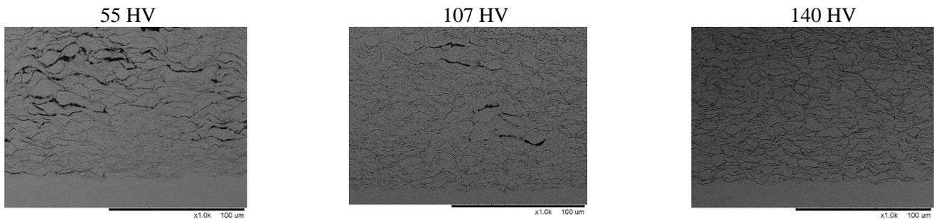
Fig. 1: SEM images of the coatings produced on the substrate with different hardness.
