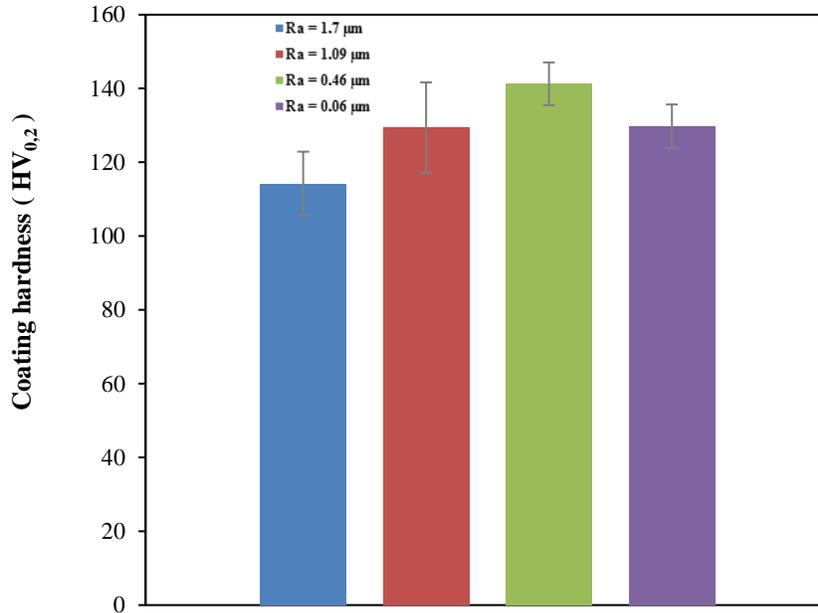
Fig. 6: Substrate surface roughness-coating hardness relation.
