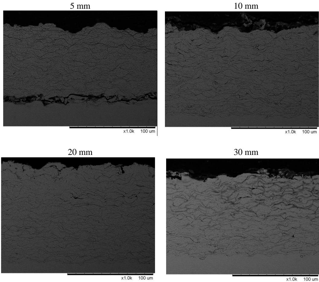
Fig. 8: SEM images of the coatings produced on the substrate with different stand-off distance.
