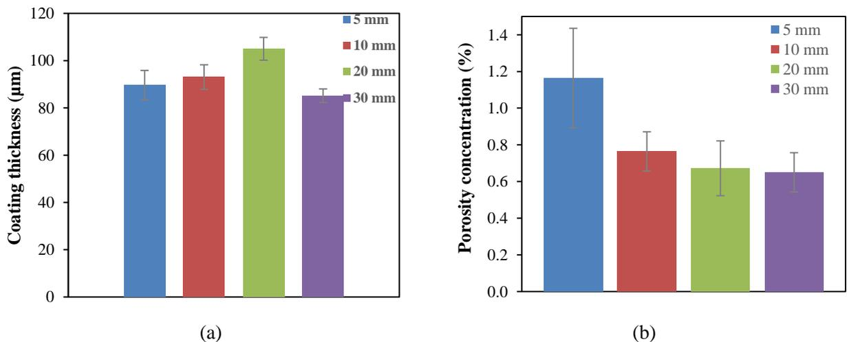
Fig. 7: (a) Stand-off distance-coating thickness relation, (b) Stand-off distance-porosity concentration relation.
