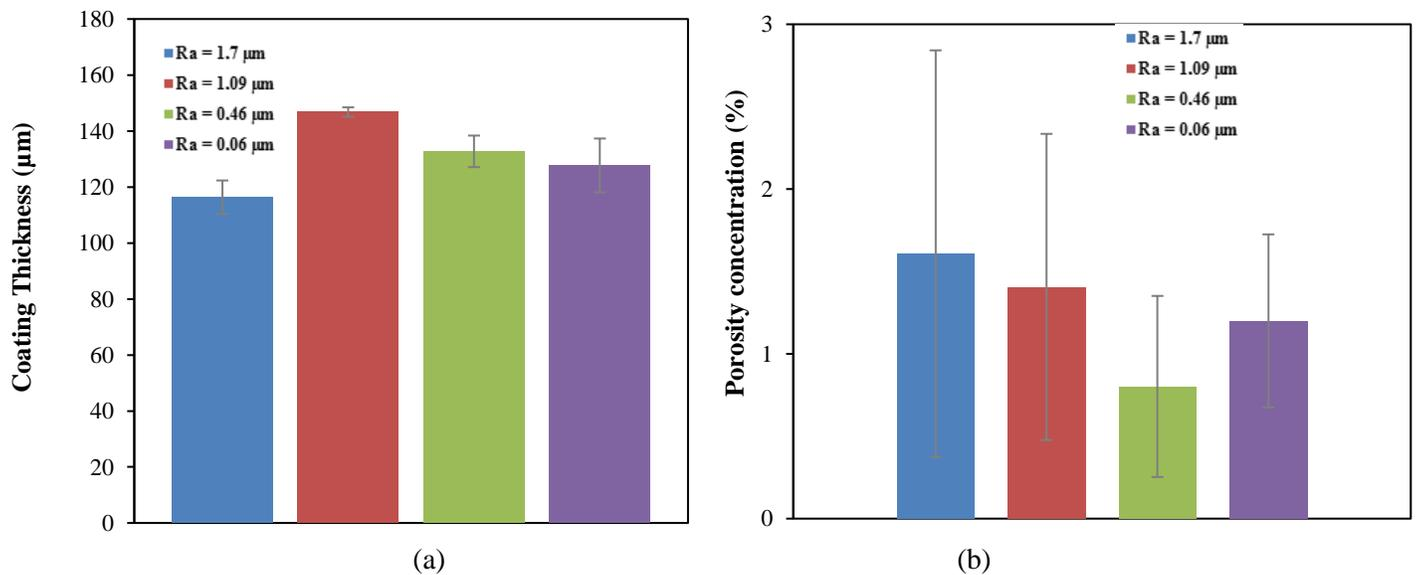
Fig. 5: (a) Substrate surface roughness-coating thickness relation, (b) Substrate surface roughness-porosity concentration relation.
