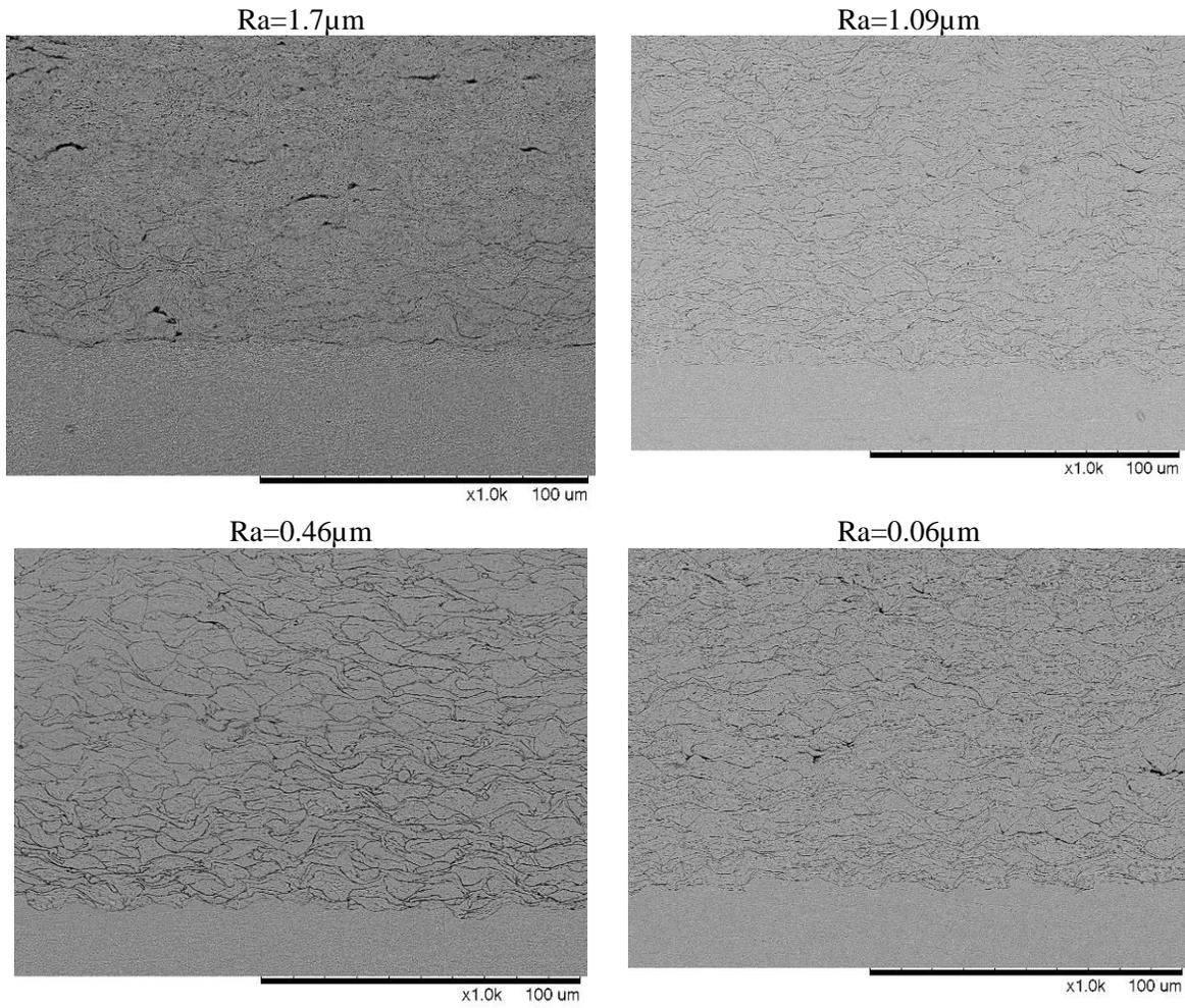
Fig. 4: SEM images of the coatings produced on the substrate with different surface roughness.
