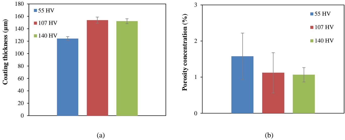
Fig. 2: (a) Substrate hardness-coating thickness relation, (b) Substrate hardness-porosity concentration relation.
