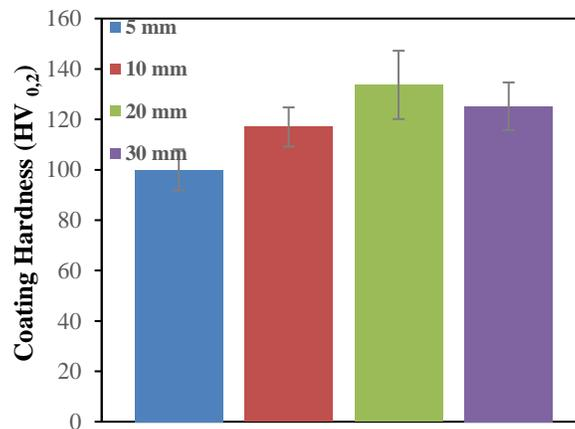
Fig. 9: Stand-off distance-coating hardness relation.
