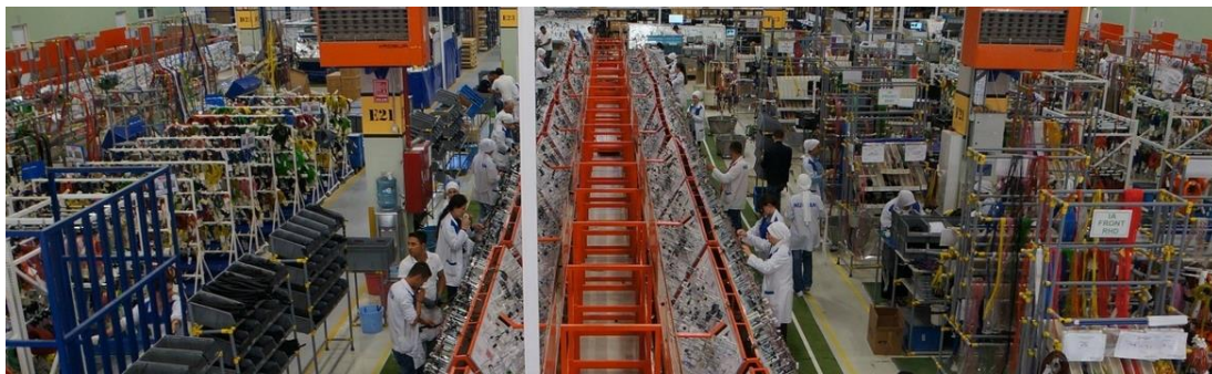
Fig. 1: Wiring harness conveyor line.
