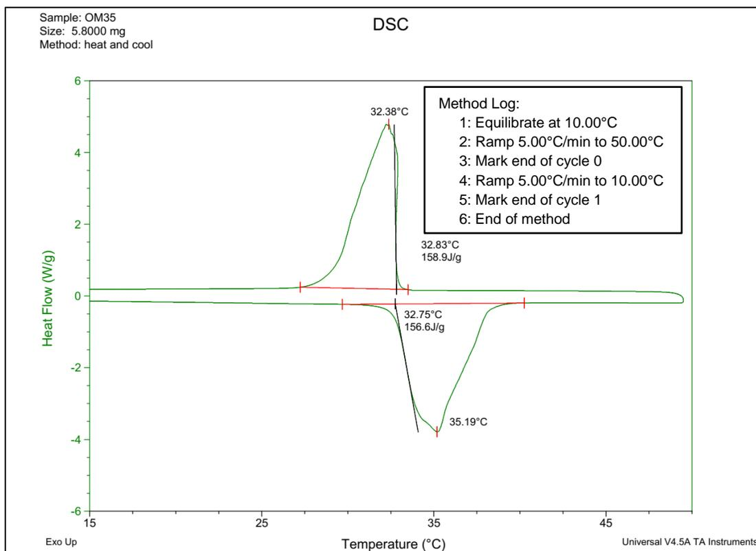
Fig. 3: Characteristic melting and solidification curve for PCM 1 (OM 35).
