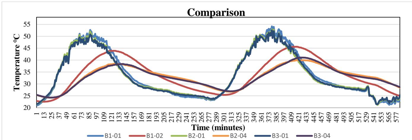
Fig. 7: Comparison of conventional and PCM incorporated bricks.
