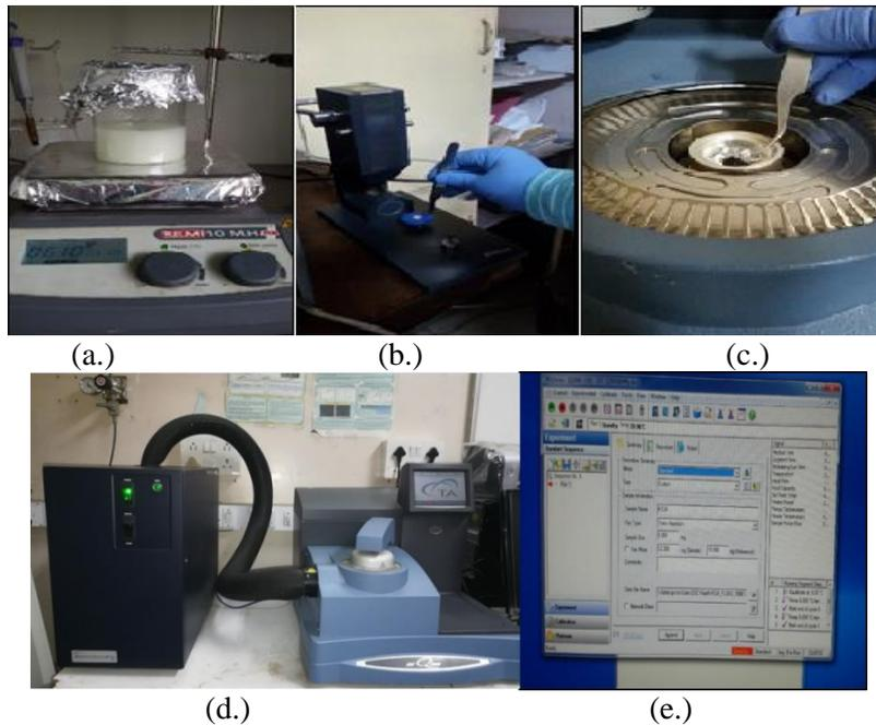
Fig. 2: (a.) PCM melting, (b.) Crimping press for PCM crimping within Tzero pan and lid, (c.) Crimped PCM sample placed in DSC cell for Testing, (d.) DSC and RCS-90, (e.) User Interface of Advantage Software v5.5.22 for data analysis.
