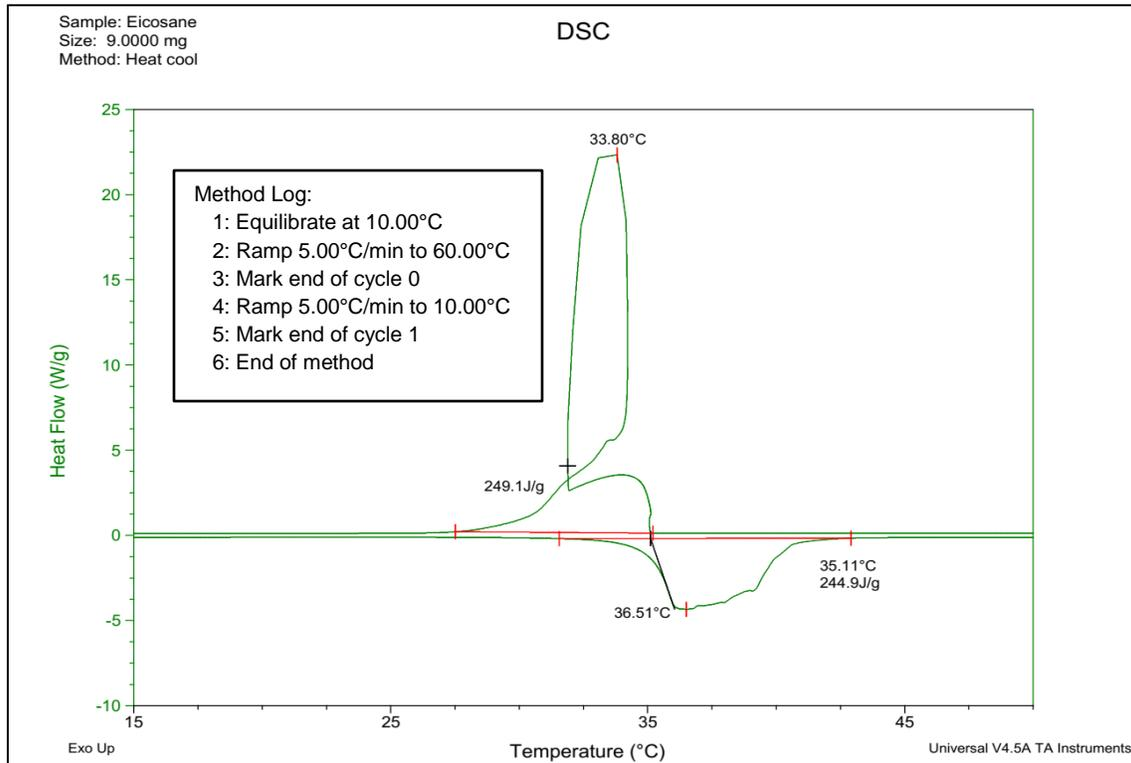
Fig. 4: Characteristic melting and solidification curve for PCM 2 (n-Eicosane).
