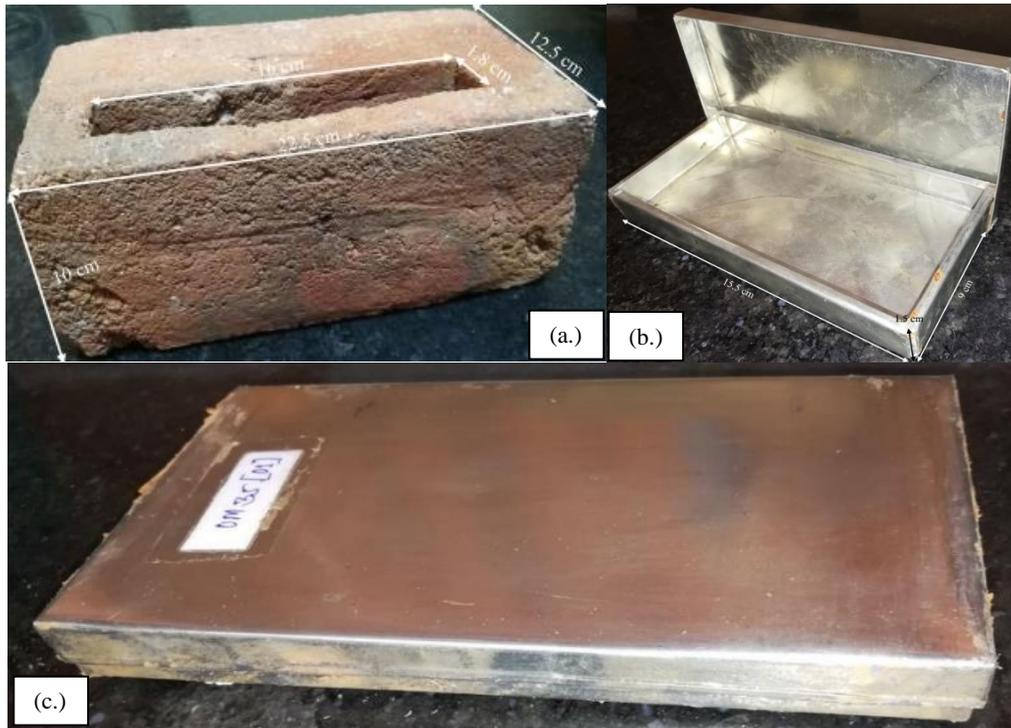
Fig. 5: (a.): Modified hollow brick; (b.): PCM encapsulating sheet metal casing; (c.): Macro-encapsulated PCM
