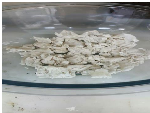
Fig. 2: The rigid polymer produced by sol-Gel method isolated from methanol.
