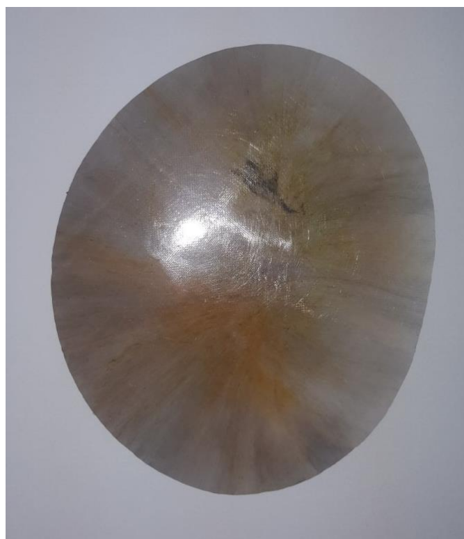
Fig. 1: The produced film from LDPE/TiO 2 /Ag NPs through the melt mixing method.
