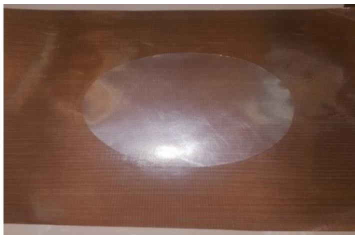
Fig. 2: The rigid polymer produced by sol-Gel method isolated from methanol.
