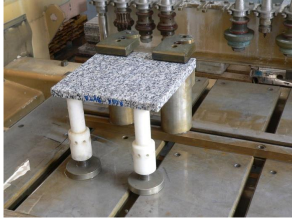
Fig. 1: Clamping of a granite table.
