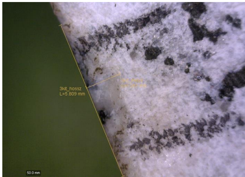
Fig. 5: Determination of an edge chipping.
