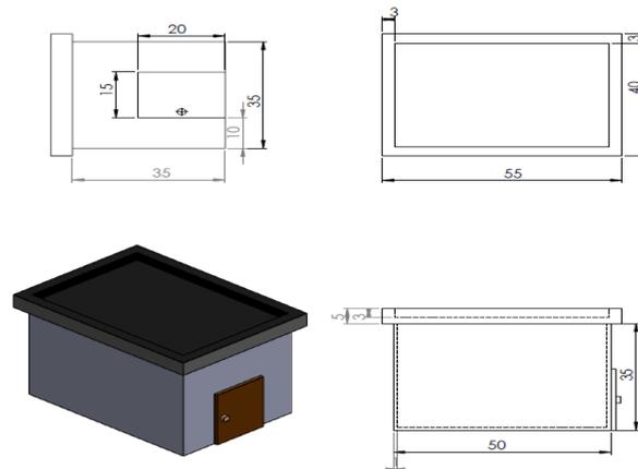
Fig. 1: Drawing sheet for the model building.
