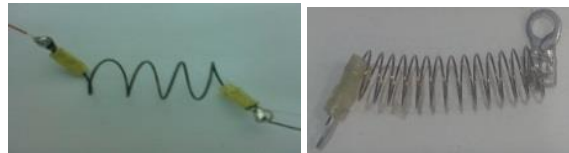
Fig. 5: Connecting helical shaped SMA element and electrical wire via crimps (metal joints).
