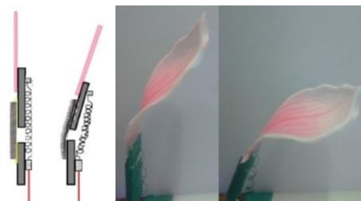
Fig. 11: the operation of the actuating mechanism for flower petal bending.
