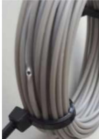
Fig. 5: The defect after burst pressure test, conditions were 80°C water bath and 48bar.
