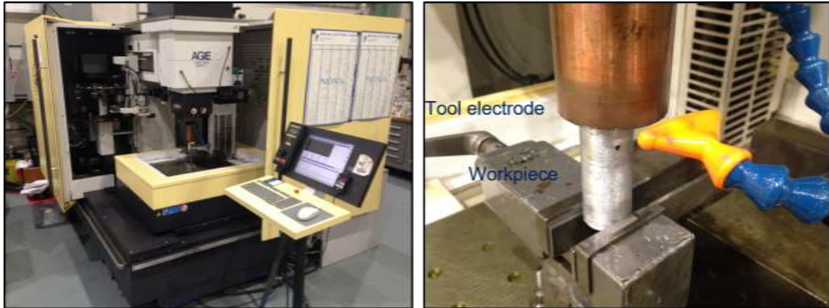
Fig. 2: Setup for Electrical discharge machining.
