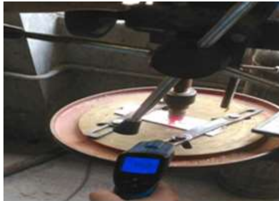
Fig. 1: Bench drilling machine showing the rotational drive and the clamping system mounted on the bed.
