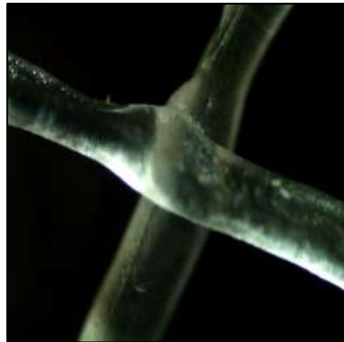
Fig. 11: Spacer after 3-hour clean with Cleaner A.
