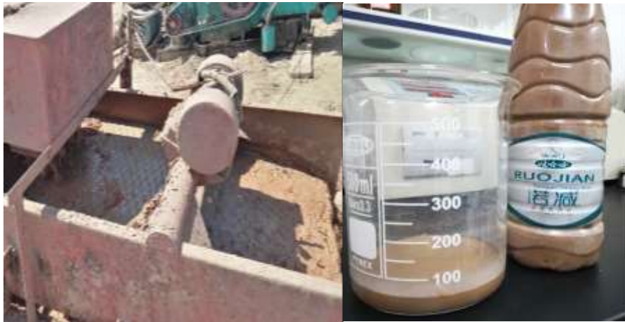
Fig. 2: Vibration desander for in-situ leaching construction site.
