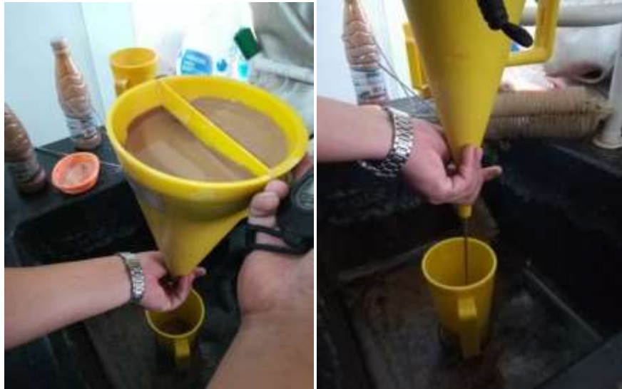
Fig. 3: Laboratory Mud Drilling Fluid Test.
