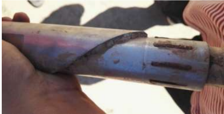
Fig. 1: Piston parts blocked by sediment.
