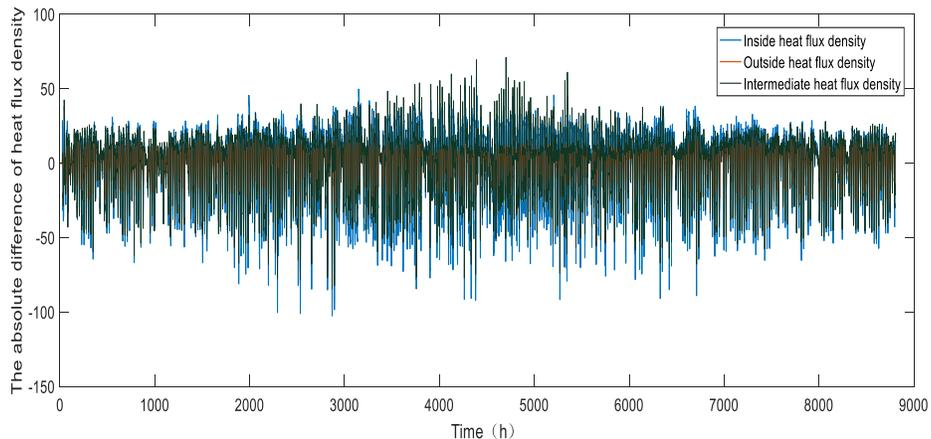
Fig.7 : Absolute difference in heat flux density between inside and outside of the Western Wall.
