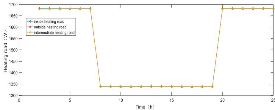
Fig. 4: Heating load in winter under three placement conditions of cement expanded perlite in typical day.
