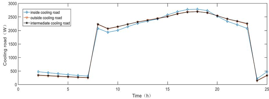
Fig. 3: Cooling load in summer under three placements of cement expanded perlite in typical day.
