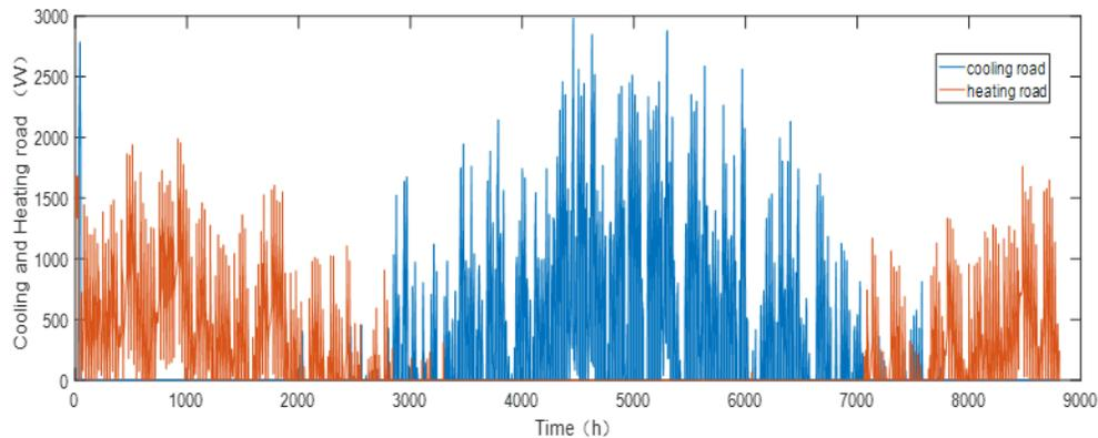
Fig. 2: Annual cooling and heating load on innermost side of cement expanded perlite with time step of 4.
