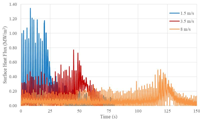
Fig. 4: Surface heat flux history when quenching a 550 °C test plate at different speeds with a water jet at 25 °C.
