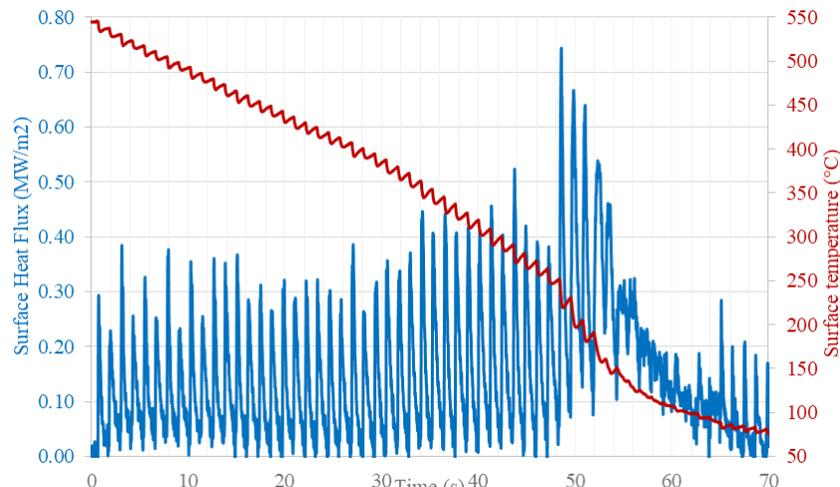
Fig. 2: Surface heat transfer and temperature estimations when quenching a 550 °C test plate moving at 3.5 m/s with a planar water jet at 25 °C.
