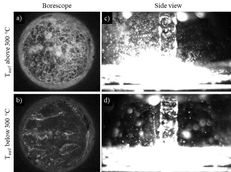
Fig. 3: Representative snapshots of high-speed recordings when quenching a 550 °C test plate moving at 3.5 m/s with a circular water jet at 25 °C.
