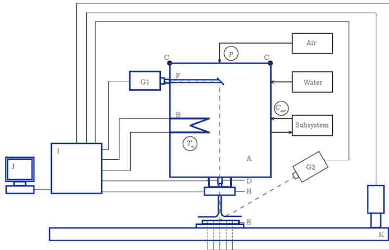
Fig. 1: Schematic representation of the experimental setup. A: Water tank. B: Heater. C: Load cells. D: Valve and nozzle. E: Test plate. F: Borescope. G1: Stagnation zone camera. G2: Side view camera. H: LEDs ring. I: Control box. J: Computer. K: Linear unit.
