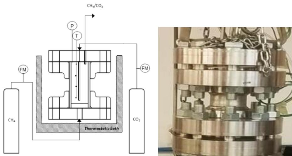
Fig. 1: Scheme of the experimental apparatus and image of the hydrate reactor.
