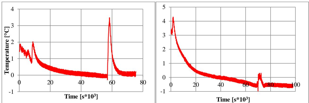
Fig. 4: Temperature trend over time in Test 3 (at left) and Test 4 (at right).
