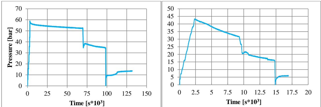
Fig. 3: Pressure trend over time in Test 1 (at left) and Test 2 (at right).
