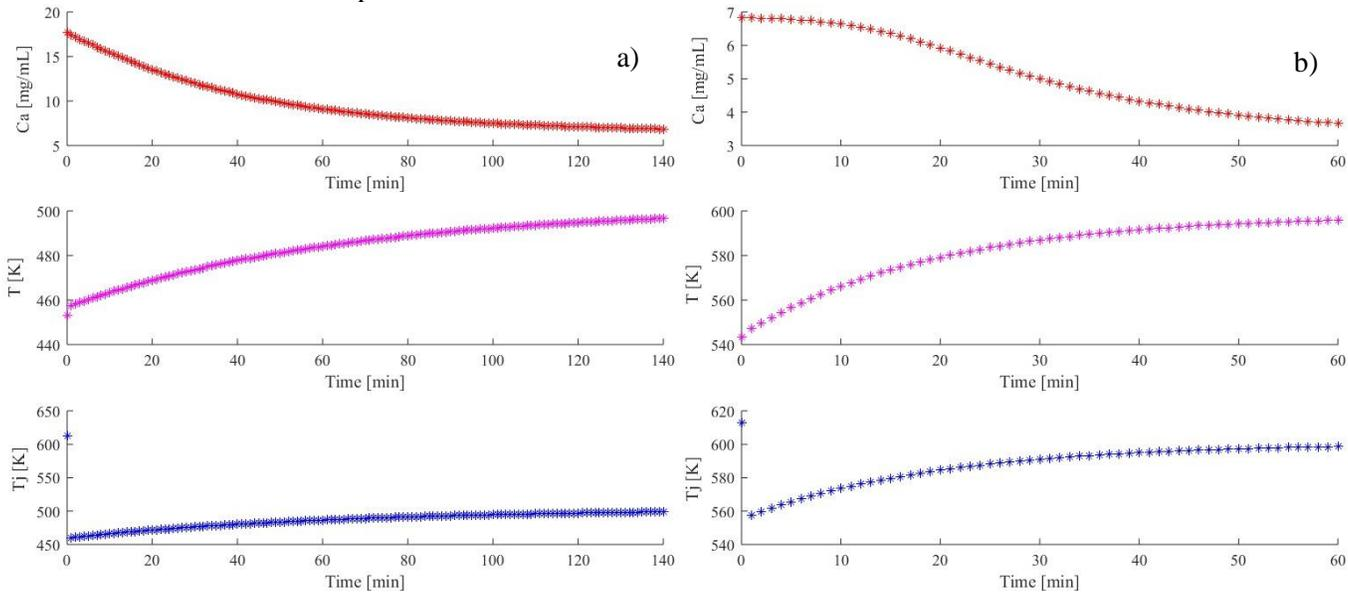
Fig. 2: Dynamic response of the reaction system at the start of the production of the MNPs. a) Nucleation phase (R-101), b) Growth phase (R-102).
