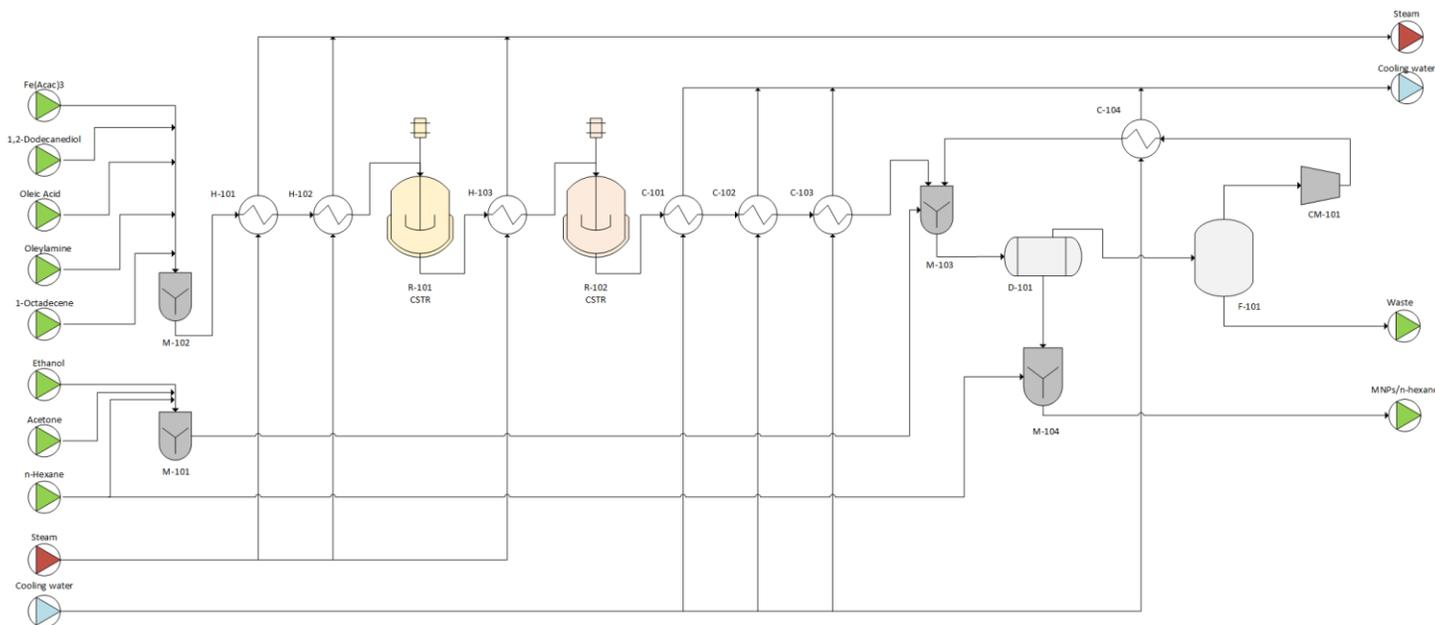
Fig. 1: Diagram of the MNPs production process by thermal decomposition.
