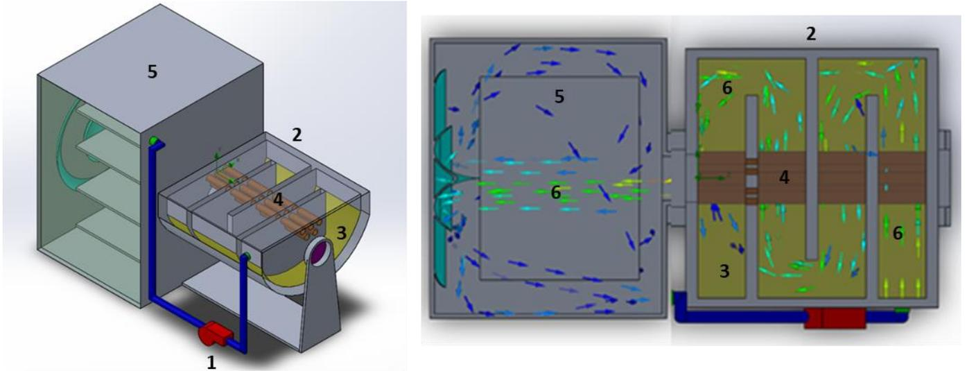
Fig. 1: Proposed design solar dryer+ Integrated Photonic Solar Reflectors and PCMs (Lateral view solar panel and air flow).
