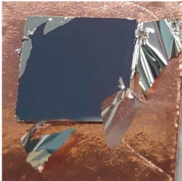
Fig. 7: Peeling test of the nano-twinned (111) Ag film with a thickness of 2 μm on a (111) Si substrate without a Ti adhesive layer.
