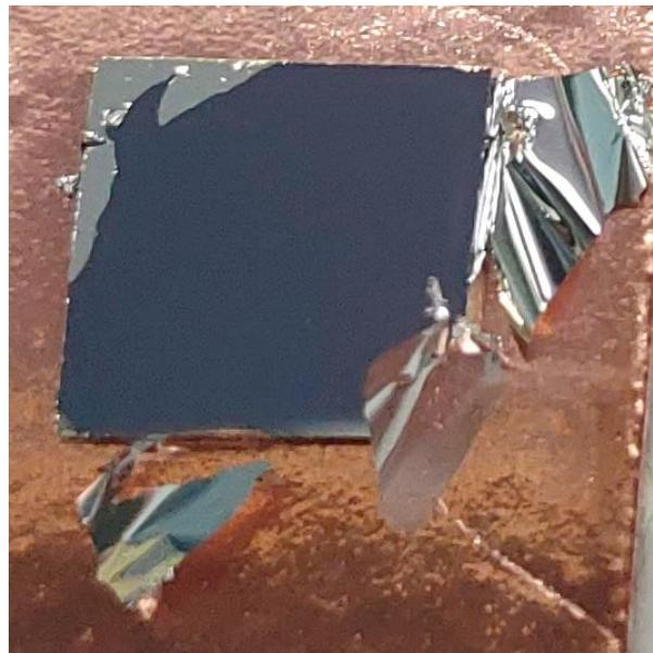
Fig. 7: Peeling test of the nano-twinned (111) Ag film with a thickness of 2  $\mu\text{m}$  on a (111) Si substrate without a Ti adhesive layer.
