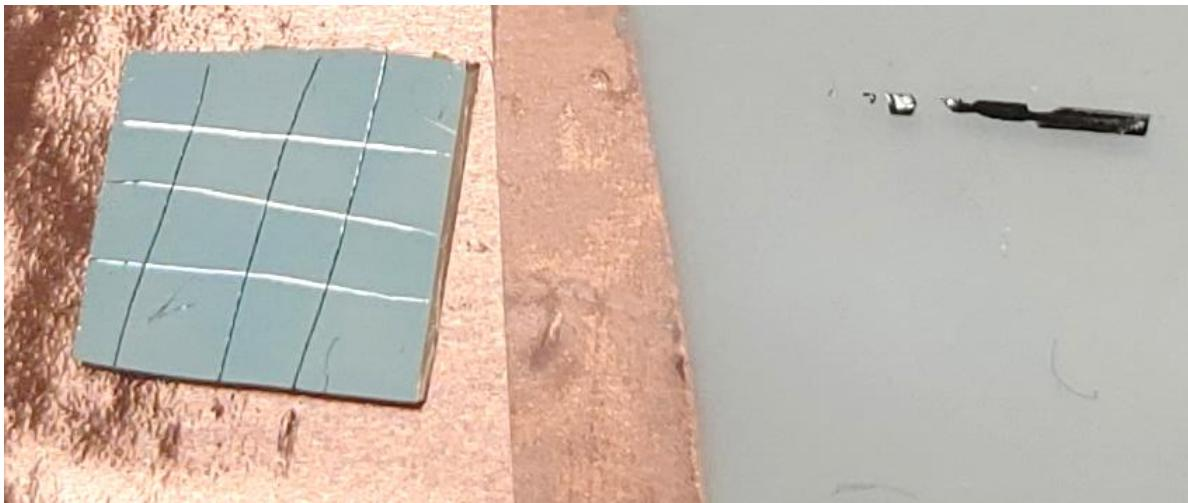
Fig. 8: Peeling test of the nano-twinned (111) Ag film with a thickness of 9  $\mu\text{m}$  on a 0.1  $\mu\text{m}$  Ti-coated (111) Si substrate.
