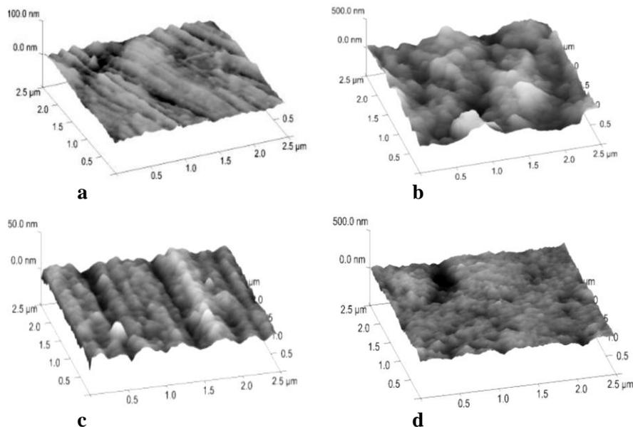
Fig. 1: AFM images of sample surfaces; **a**: bare metal, **b**: bare metals surface after immersion in 3,0 m/m% NaCl solution for 1 h; **c**: bare metal covered by undecenyl phosphonic acid SAM layer; **d**: the undecenyl phosphonic acid SAM layer-covered carbon steel surface after immersion into 3,0 m/m% NaCl solution for 1 h [11].
