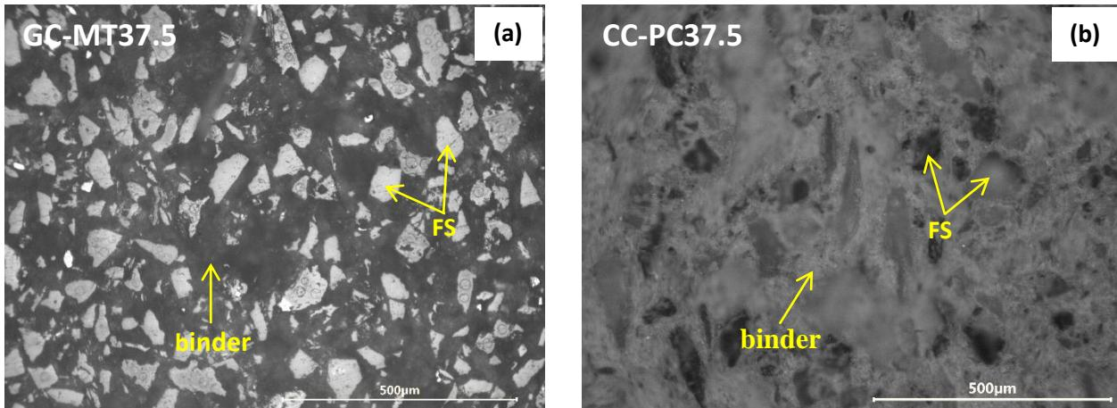
Fig. 3: Optical microscopy micrographs of polished surfaces of (a) GC-MT37.5 and (b) CC-PC37.5.
