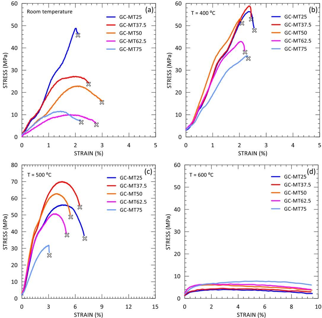
Fig. 5: Stress-strain curves of GC samples tested at (a) room temperature, (b) 400 °C, (c) 500 °C and (d) 600 °C.
