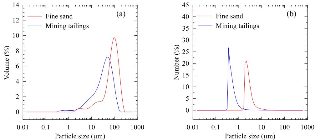
Fig. 1: Particle size distribution in (a) volume and (b) number for MT (blue line) and FS (red line).
