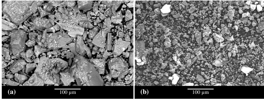
Fig. 2: SEM micrographs of (a) FS and (b) MT.
