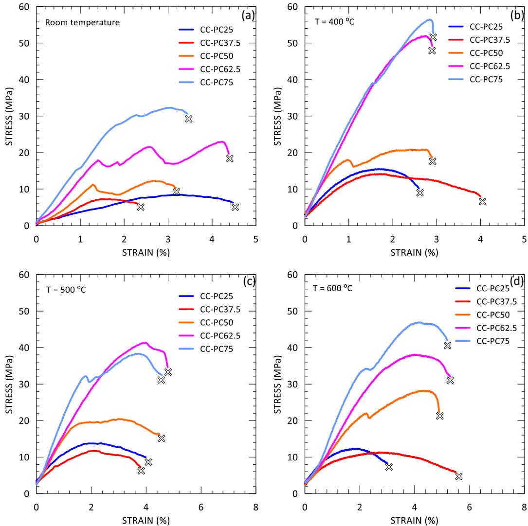
Fig. 6: Stress - strain curves of CC samples tested at (a) room temperature, (b) 400 °C, (c) 500 °C and (d) 600 °C.
