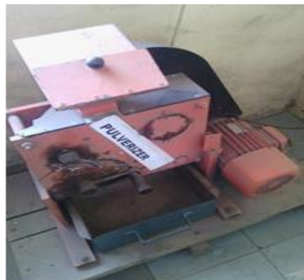
Fig 1: FRITSCH laboratory jaw crusher Pulverisette used for Comminution
