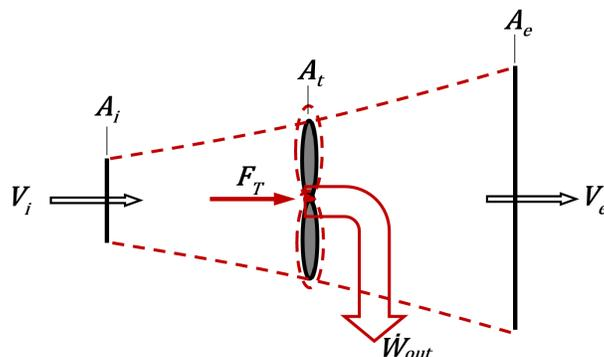
Fig. 1: Diagram of stream tube used in the application of linear momentum theory.
