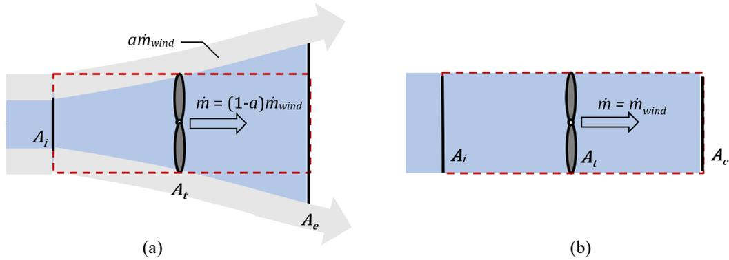
Fig. 4: (a) For any  $a > 0$ , a fraction of  $\dot{m}_{wind}$  is deflected around the actuator disc. (b)  $\dot{m} = \dot{m}_{wind}$  only when  $a = 0$ , which corresponds to zero power output.
