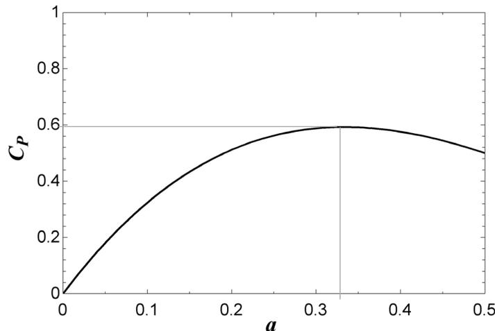
Fig. 2: Relationship of power coefficient to axial induction factor according to linear momentum theory. The maximum value of  $C_P$  is  $16/27$  and occurs at  $a = 1/3$ .
