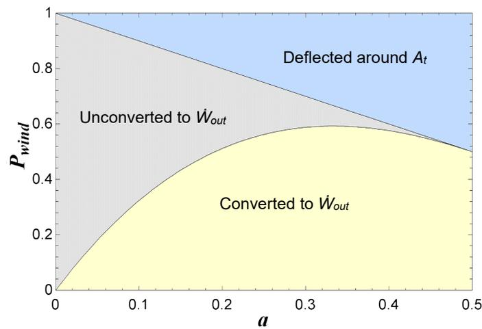
Fig. 5: Relative proportions of  $P_{wind}$ . The blue area is the fraction of  $P_{wind}$  that is deflected around the actuator. Of the power delivered to the actuator, the yellow area is the fraction converted to power output whereas the grey area remains unconverted, ultimately exiting through  $A_e$ .
