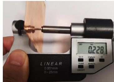
Figure 3 The thickness of an ultrathin vapor chamber after evacuation and charging process
