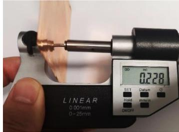
Figure 3 The thickness of an ultrathin vapor chamber after evacuation and charging process
