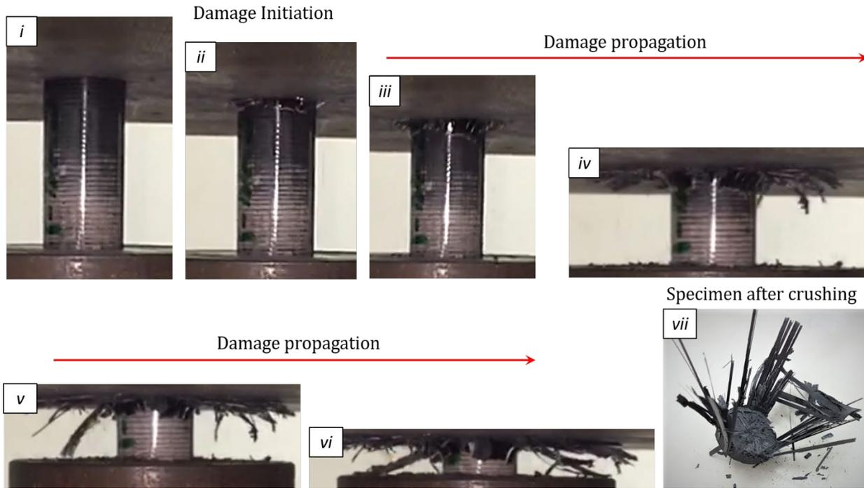
Fig. 2: Crushing mechanism of the CFRP composite tube.
