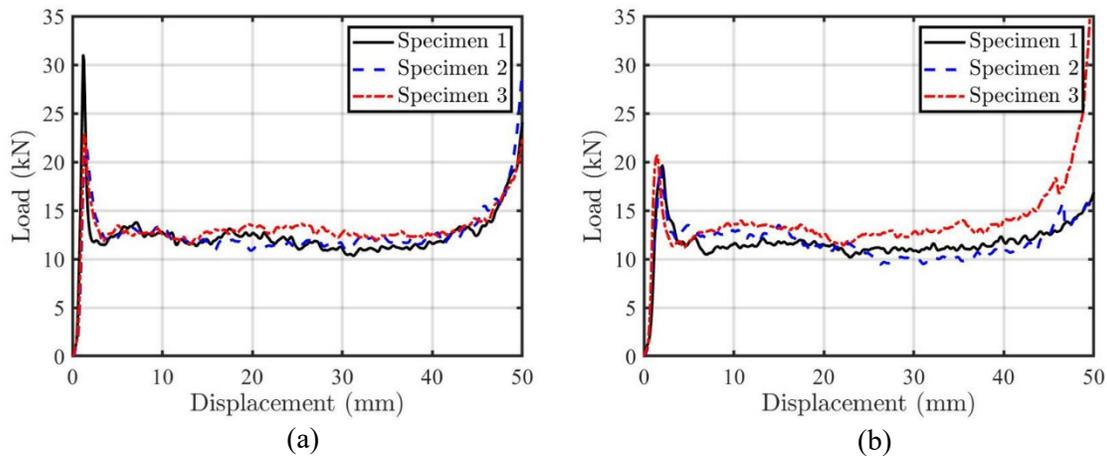
Fig.1: Load-displacement profile of the specimens (a) without thermal aging and (b) with thermal aging at 120 °C. Three samples are shown for each condition.
