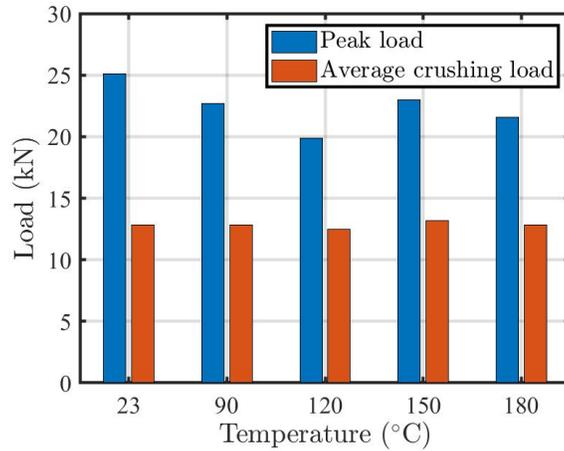
Fig. 4: Peak and average crushing force as functions of the aging temperature.
