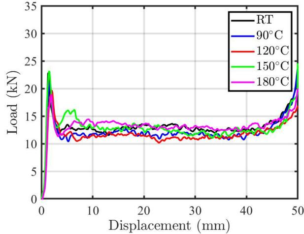
Fig. 3: Summary of the effect of the aging temperature on the load-displacement profile of the CFRP composite tubes.
