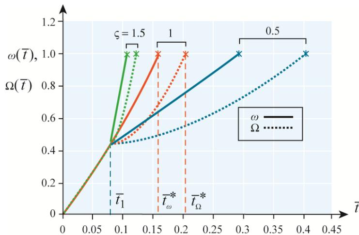
Fig. 2: Damage versus time for scalar and vector approaches.
