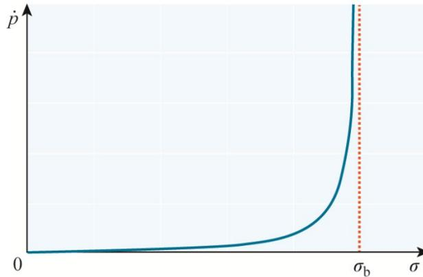
Fig. 1: Linear fractional dependence of the creep strain rate on stress at  $\sigma_0 = 0$ .
