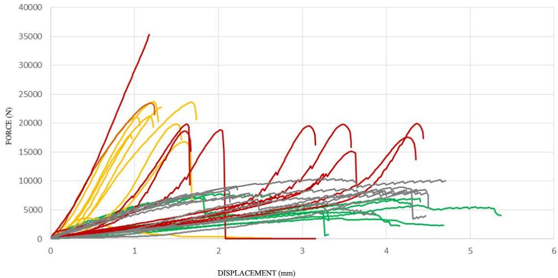
Fig. 2: Load-displacement relationship of the 10 specimens V13 (red), V12 (yellow), V23 (gray) and V32 (green)
