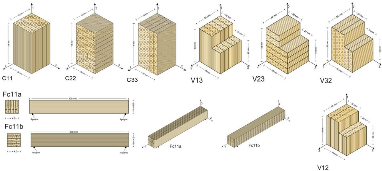
Fig. 1: C11 / C22 C33 specimens for compression test; V13 / V23 / V32 specimens for tensile test; Fc11a / Fc11b Bending Test Specimens, ASTM D143.
