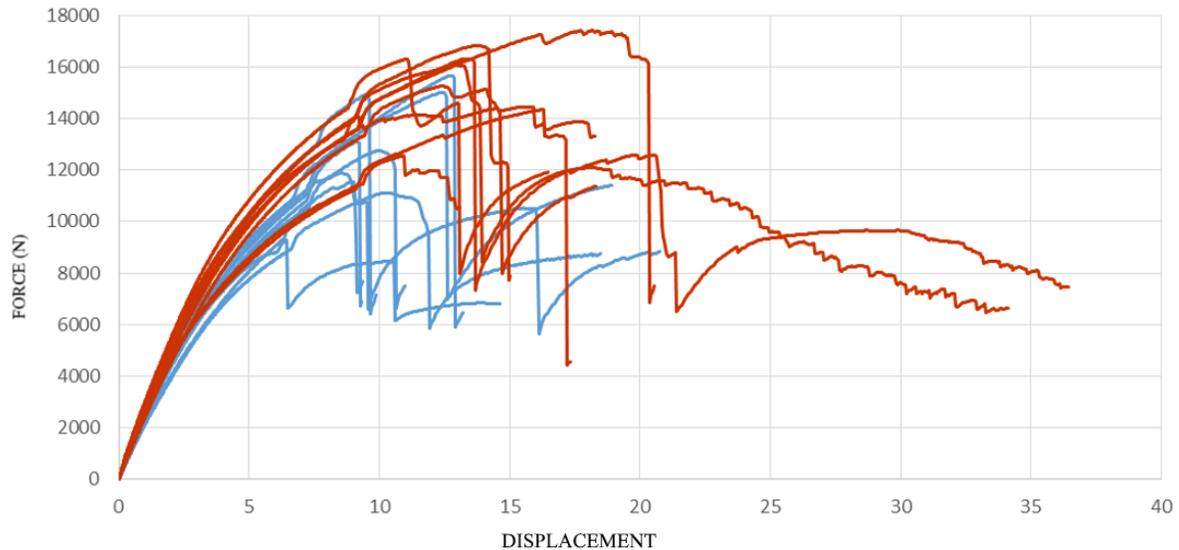
Fig. 3: Load-displacement relationship of the 9 specimens Fc11a (red) and the 9 specimens Fc11b (blue).
