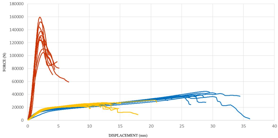
Fig. 2: Load-displacement, 10 specimens C11 (red), the 9 specimens of C22 (blue) and the 10 specimens C33 (yellow)
