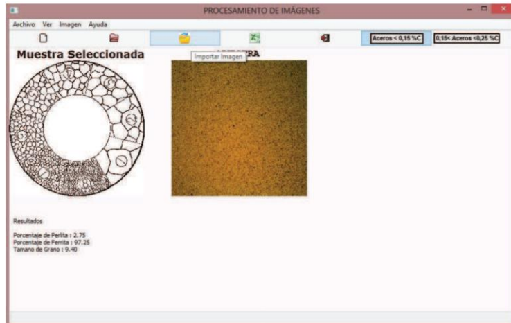
Fig. 3: Graphical interface metallographic software developed with Python.
