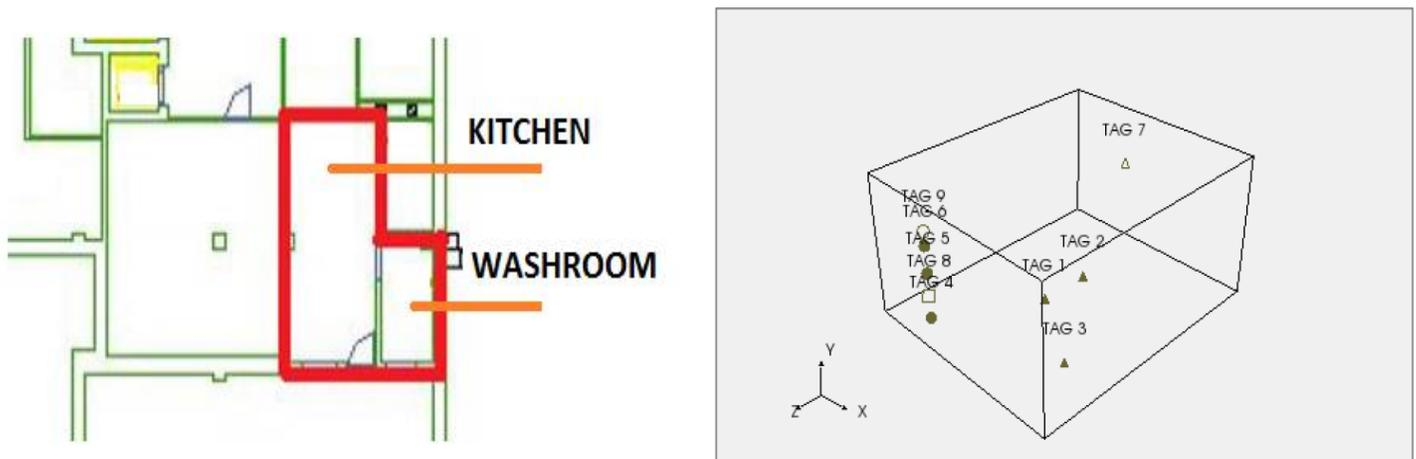
Fig. 1: The position of the kitchen and the location of the probes in the program Dantec ComfortSense
