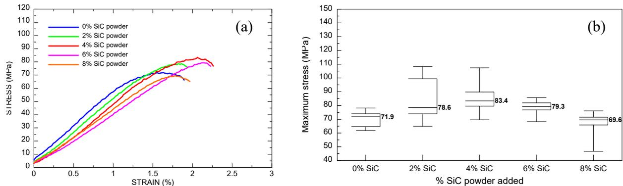
Fig. 3: (a) Stress vs. strain curves for the five types of mortars studied, (b) relationship between the maximum stress and the percentage of SiC powder added.
