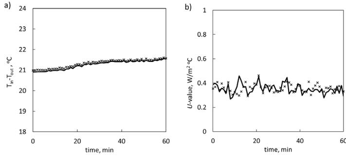
Fig. 1: Time variations of a) inside and outside temperature difference, and b) overall heat transfer coefficient for the case of an insulated system with polystyrene cover on the top of each box. Lines and crosses correspond to measurements in each hot-box.
