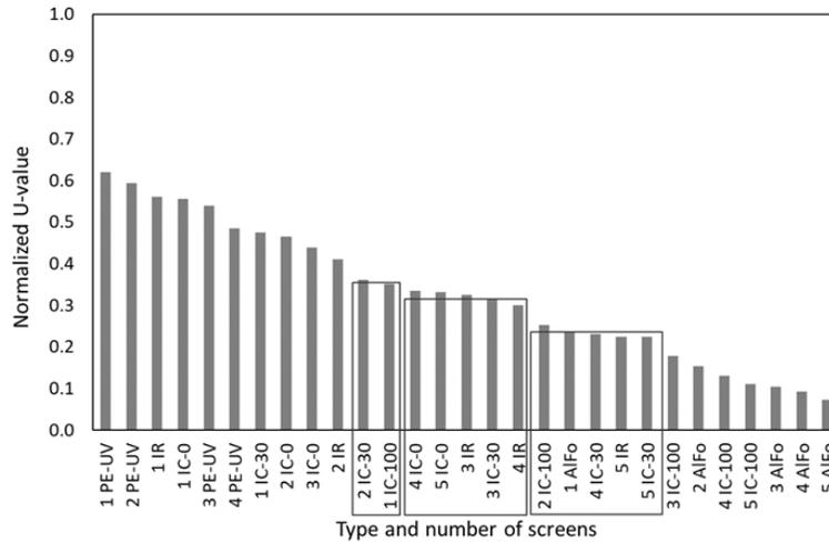
Fig. 3: Measured overall heat transfer coefficients for the IR blocking covering polyethylene in combination with one to five layers of different types of thermal screens (PE-UV, IR, IC-0, IC-30, IC-100, AlFo). The values were normalised using the value for IR cover without screens ( $U_{IR\ cover} = 7.44\ W\ m^{-2}\ ^\circ C^{-1}$ ,  $\sigma = 0.39$ ). Rectangles showing along with x-axis denote screening combination with similar normalised  $U$ -values.
