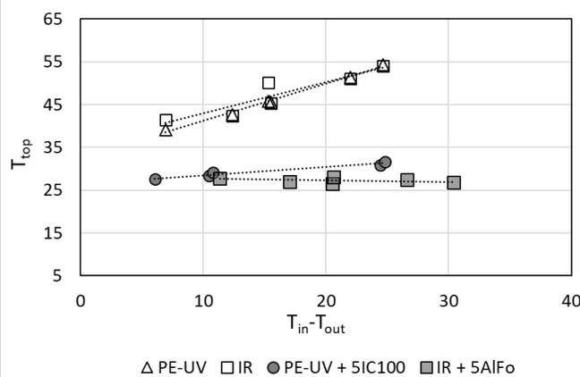
Fig. 4: The temperature of the air underneath a cover material installed at the top of the hot box.
