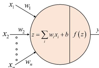
Fig. 1: Schematics of mathematical model for a single neuron.
