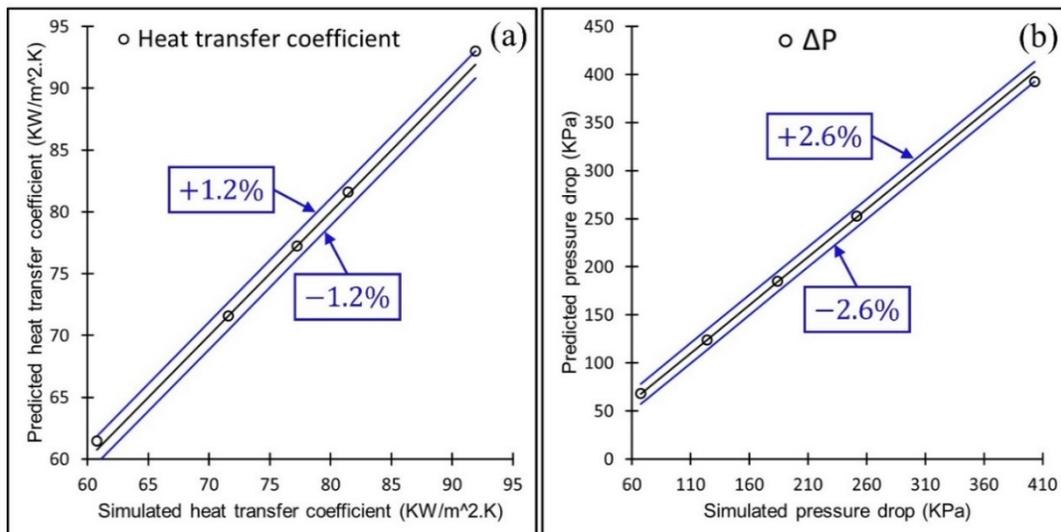
Fig. 5: Comparison between predicted and simulated values: (a) heat transfer coefficient; (b) pressure drop.
