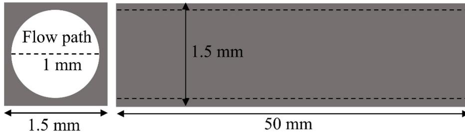
Fig. 2: Schematic of the cold plate.
