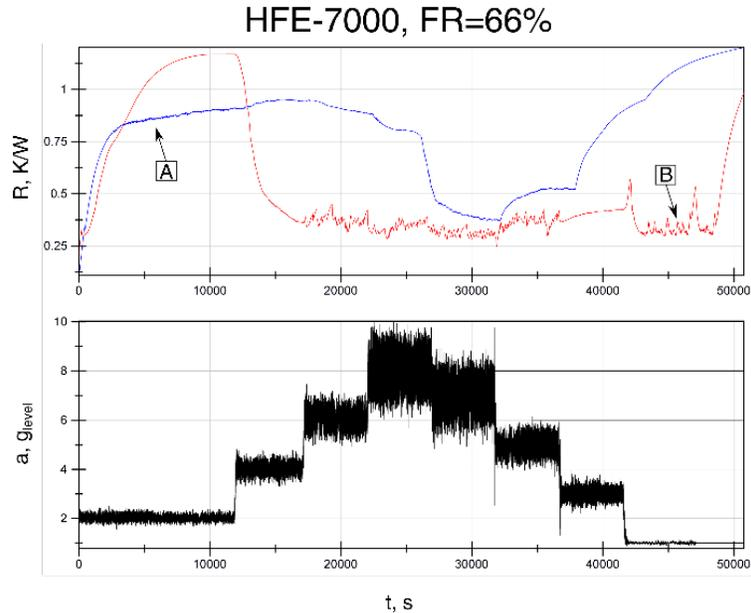
Figure 3 Thermal resistance and acceleration as a multiplication of normal acceleration in the Earth's gravitational field for low boiling point fluid with 66% of filling ratio..
