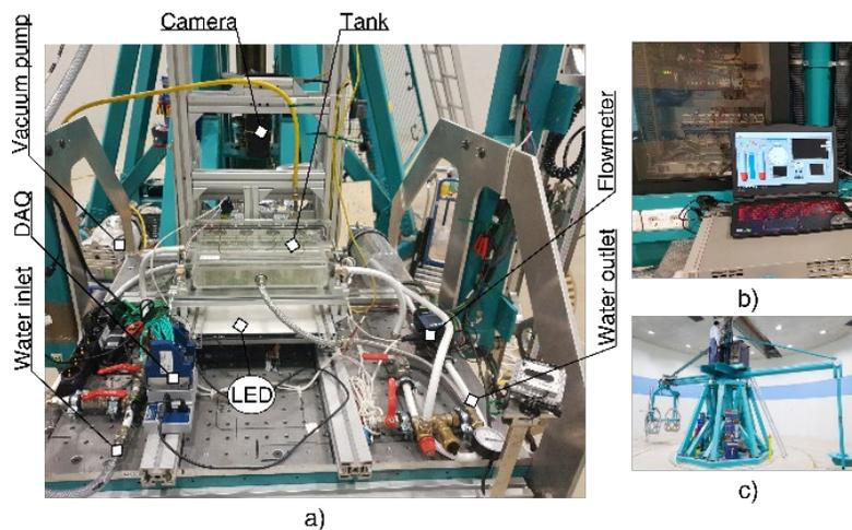
Figure 2 Main view of a) test stand, b) central control platform, c) Large Scale Centrifuge.
