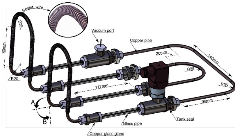
Figure 1 CAD model of tested PHP.
