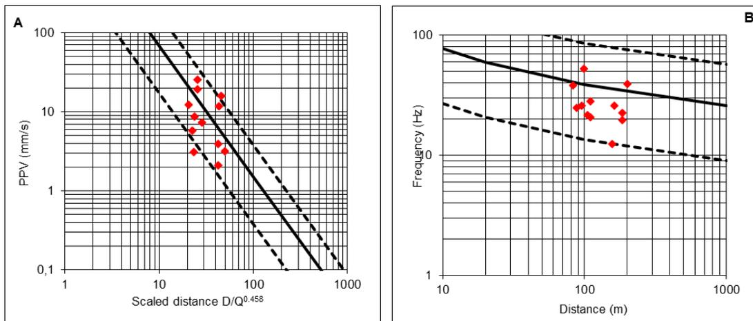
Figure 5: Limestone attenuation laws for PPV and frequency and recorded values from the real blasts.
