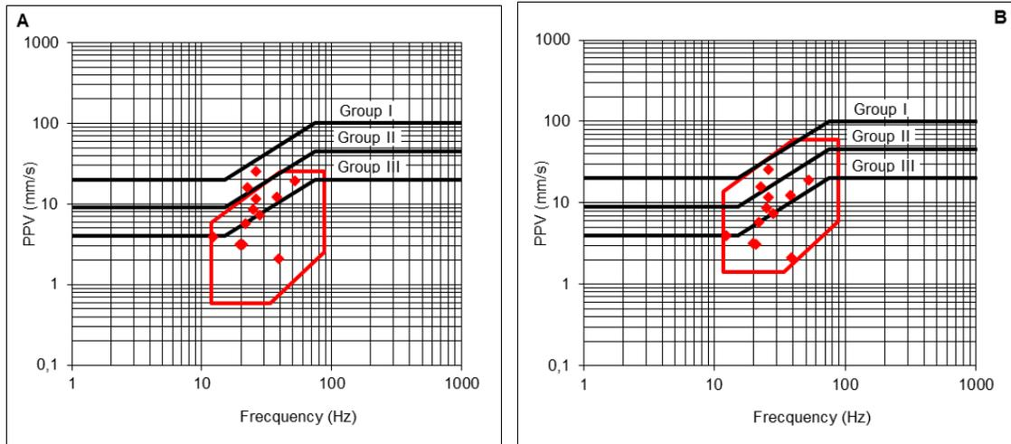
Figure 4: Representative areas predicted and actual data from real blasts in the damage prevention abacus.
