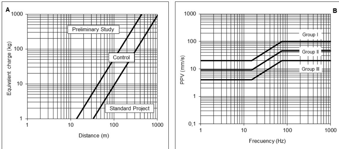
Figure 1. Abacus to determine the type of study and abacus with damage prevention criterion after Spanish Standards.
