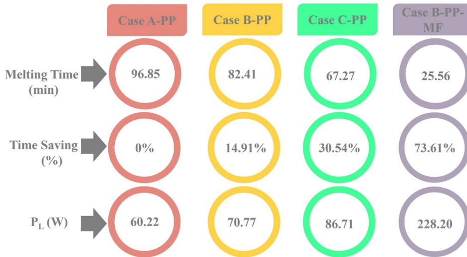
Fig. 6: A comparison between all cases with PP and metal foam: melting time, time saving and heat transfer rate
