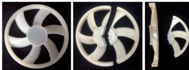
Fig. 1: Fan with hallow blades and shroud ring [8].
