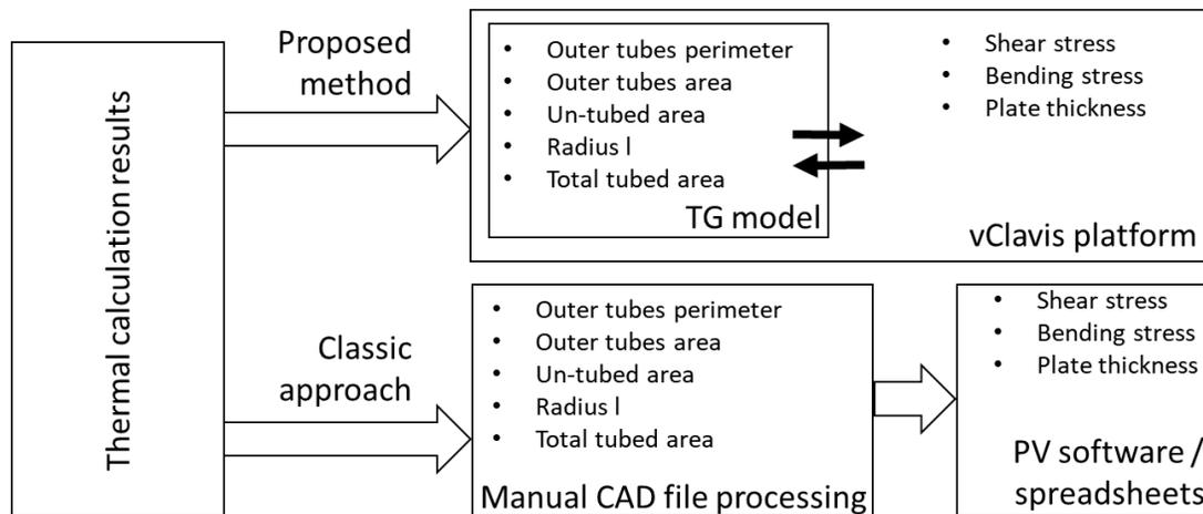
Fig. 2: Process flow comparison of the proposed model integration in PV software compared to the current status quo in the industry
