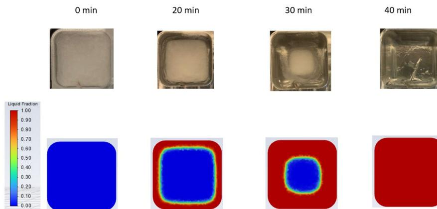
Figure 10: Liquid fraction contour comparison for A58H.
