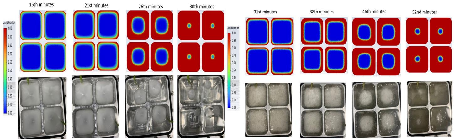
Figure 9: Liquid fraction contour comparison for RT-65 (left) and S72 (right) PCMs.
