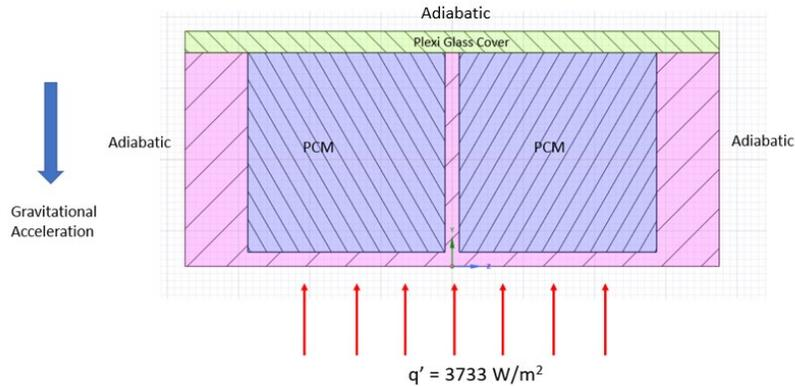
Figure 5: Boundary conditions of numerical model.
