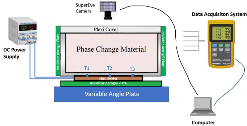
Figure 2: Schematic of the experimental setup.
