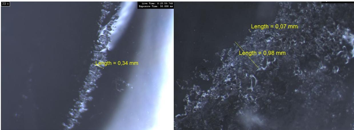
Figure 7: Dendrites of RT-65 and S72 PCMs.
