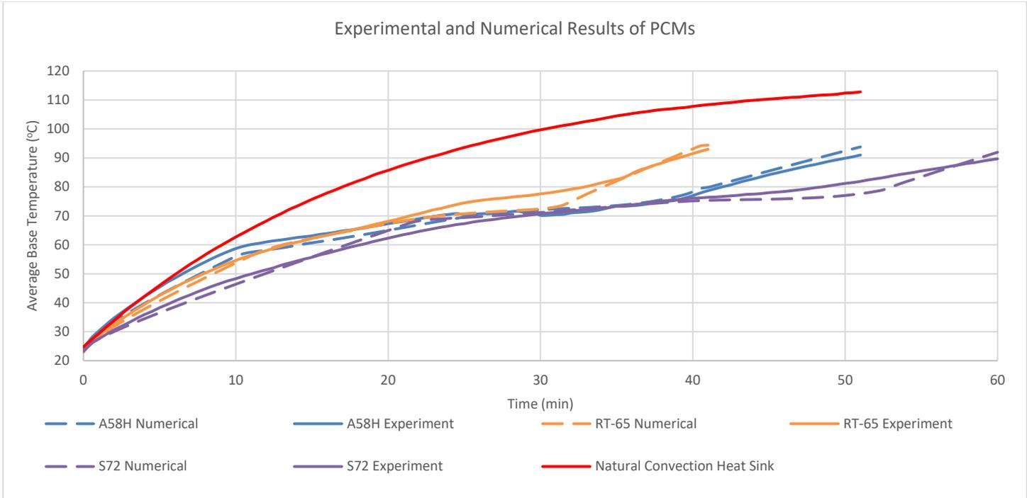
Figure 8: Experimental and numerical results of PCMs.
