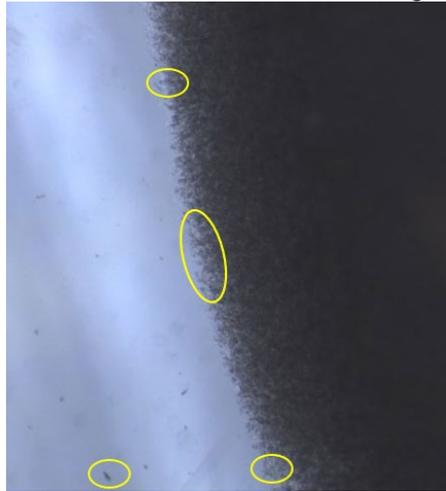
Figure 6: Dendrites of A58H PCM.
