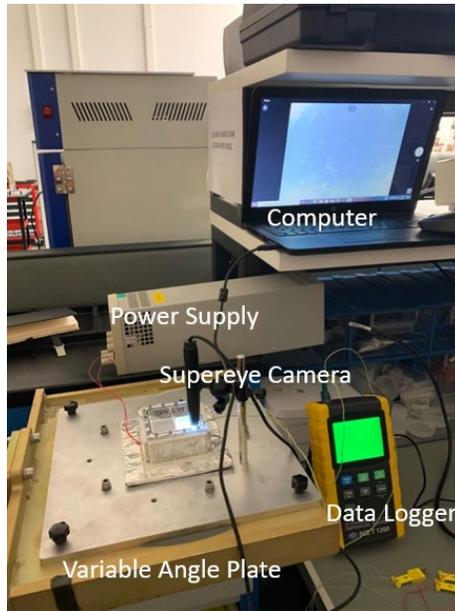
Figure 3: Experimental setup.
