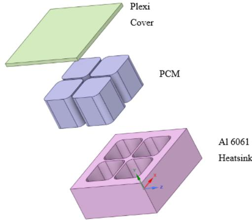
Figure 4: Numerical model of PCM heatsink.
