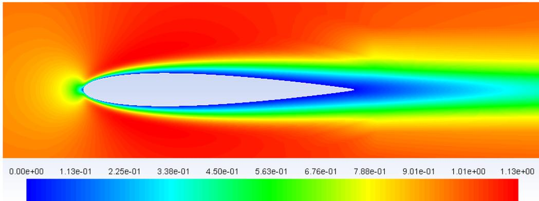
Fig. 6: Velocity contour for a zero angle of attack.
