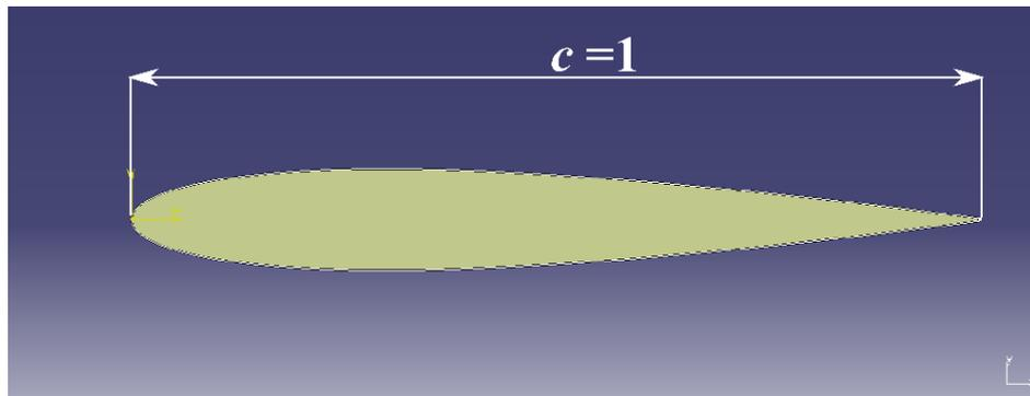
Fig. 1: Airfoil NACA 0012 description.
