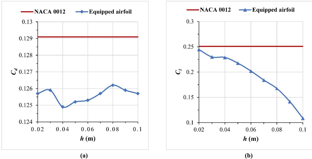
Fig. 8: Evolution of the aerodynamic coefficients with the device height  $h$ .
