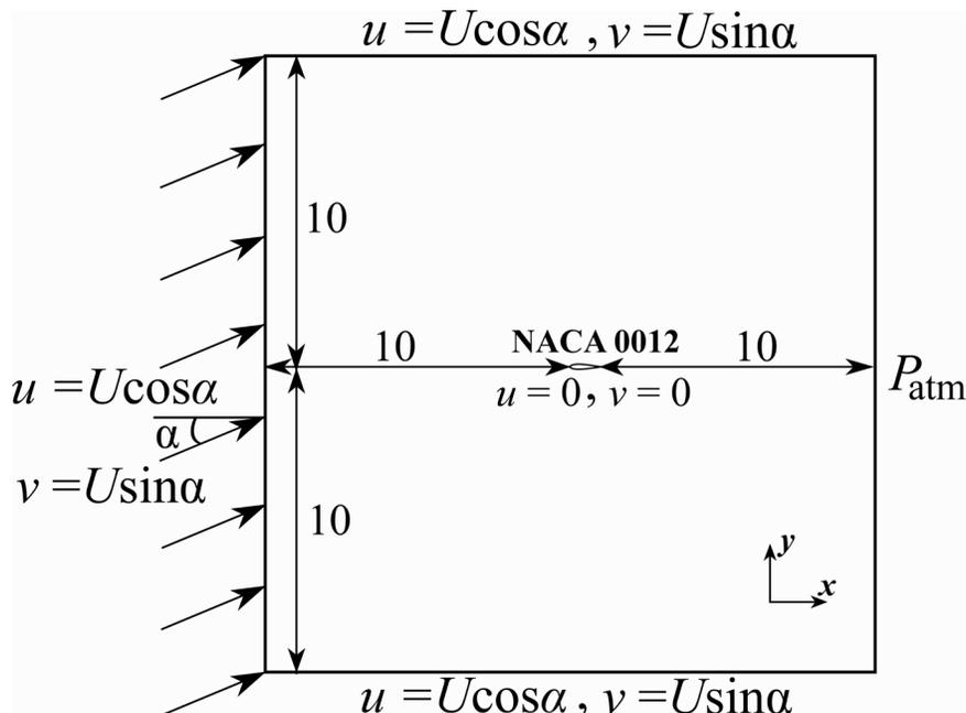
Fig. 3: Boundary conditions of current simulations.
