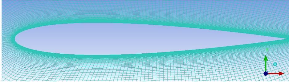
Fig. 4: Non-uniform structured mesh used in this study.
