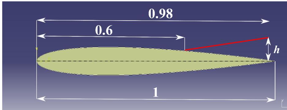
Fig. 2: Emplacement of the device of drag reduction.
