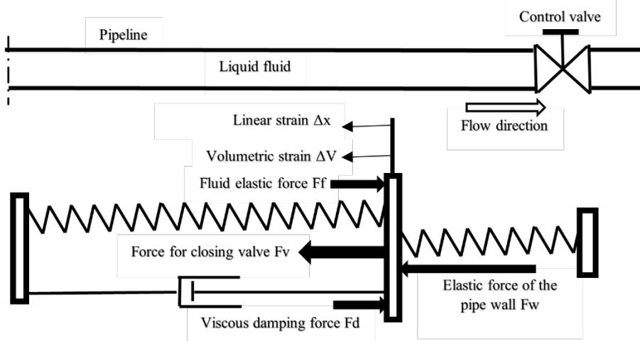
Fig. 2: Representation of a hydraulic installation as a mechanical target process.
