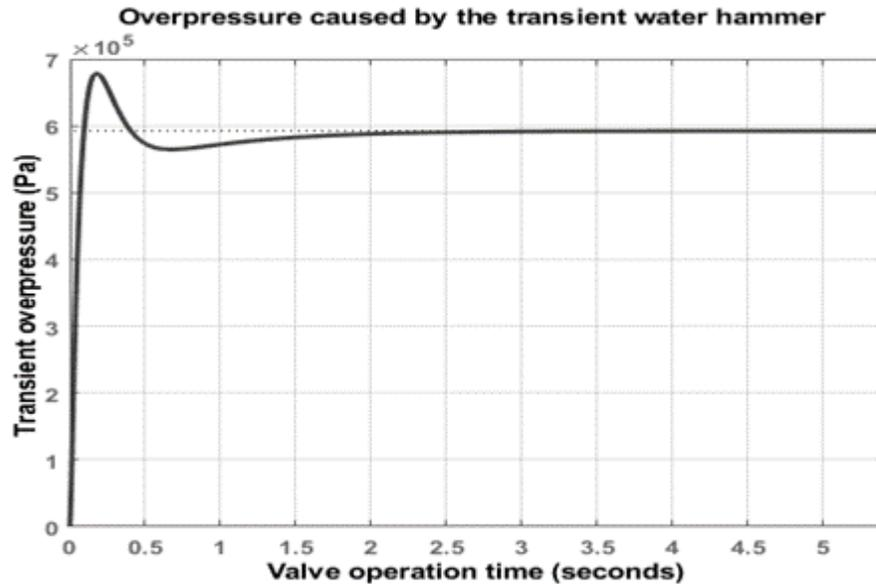
Fig. 4: Overpressure caused by the transient water hammer.
