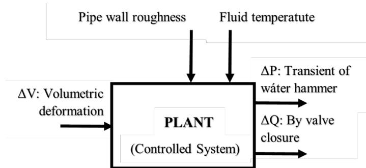
Fig. 1: Inputs, outputs, and disturbances of the hydromechanical installation.
