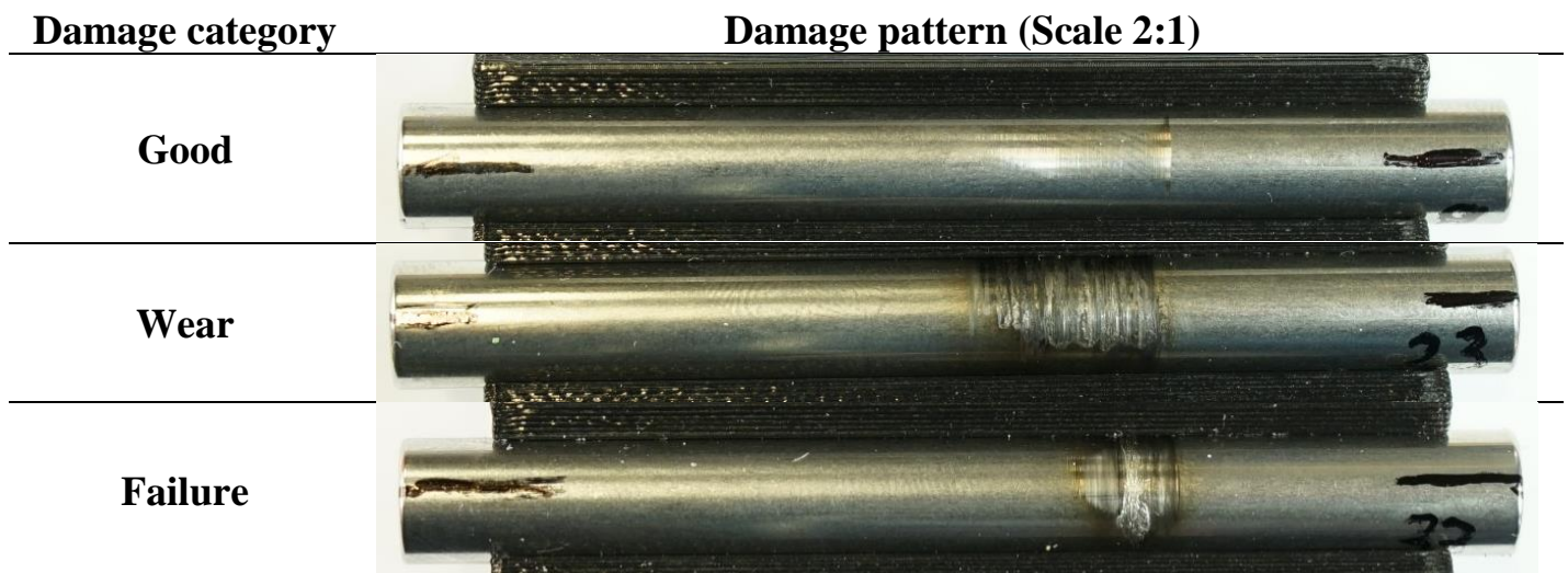
Fig. 3: Illustration of the three damage categories "Good" (top), "Wear" (middle) and "Failure" (bottom)
