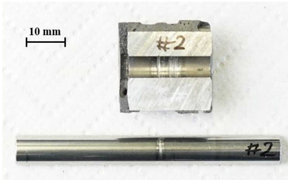
Fig. 5: Scuffing damage on test bushing (top) and test shaft (bottom)
