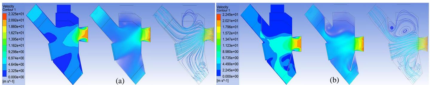
Figure 2: Ansys Fluent simulations on the preliminary design (a) Iteration 1; (b) Iteration 2
