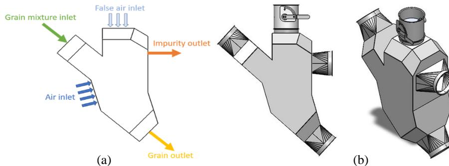
Figure 1: (a) Grain aspirator concept; (b) Preliminary design of the grain aspirator
